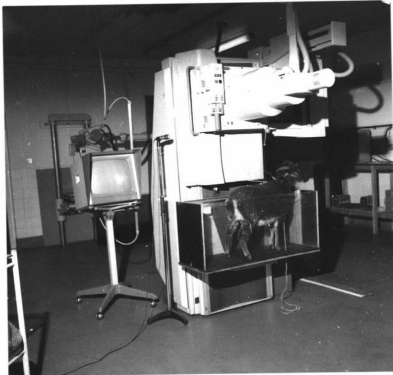
At the output of the image intensifier was a two way image splitter which allowed the mounting of either a 35 mm cine-camera or a 70 mm spot-film camera.
