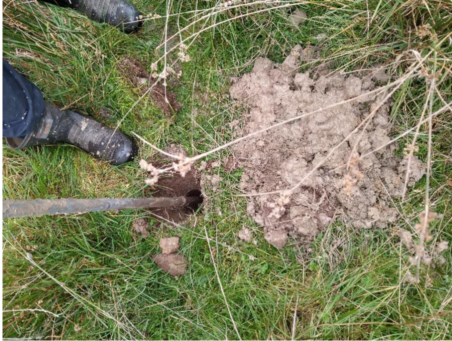
Figure 23: An auger hole for piezometer instillation using a one-piece Dutch auger.
