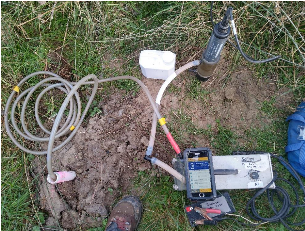
Figure 31: The equipment used for the sampling of groundwater. Top right - YSI Flowcell Sensor with sample collection bottle to the left. Bottom left - pipes in the piezometer and connected to the pump for the removal of water. Bottom right - Solinst Peristaltic Pump attached to battery with cell phone on top displaying live updates from the YSI Flowcell Sensor.
