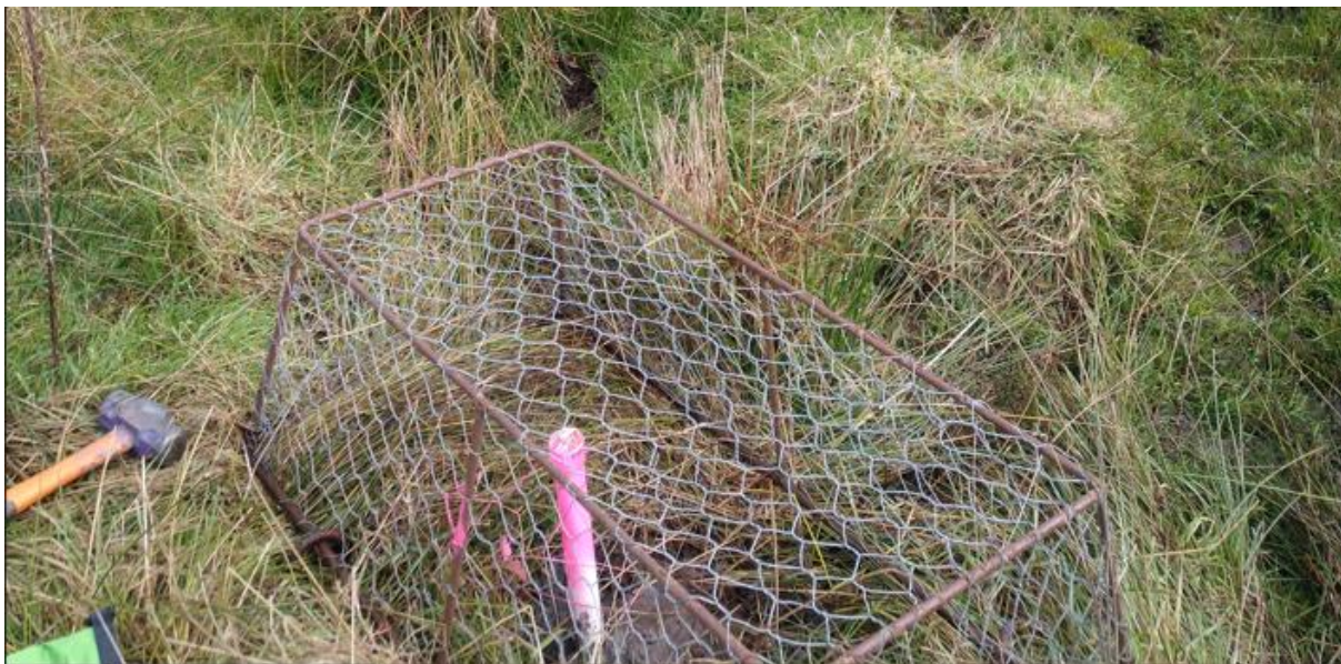
Figure 26: The instillation of a pasture exclusion cage around a piezometer (piezometer sprayed pink for identification within the field).
