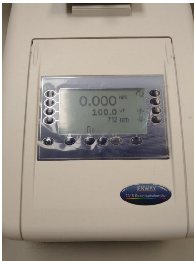
Figure 35: The screen of the Jenway 7315 Spectrophotometer with the 712nm absorbance peak used for analysing water samples for DRP.
