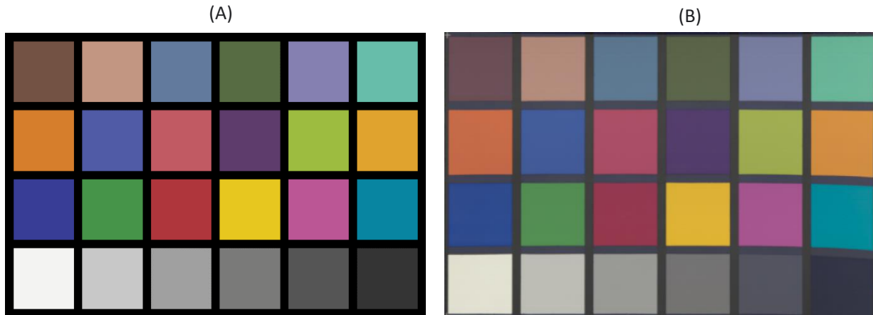
Figure 3.23: Comparison of computer generated (A) (Image Analyst, 2022) and estimated (B) X-Rite ColorChecker
