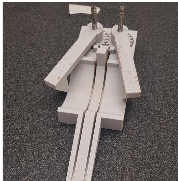
Figure 3.3: 3D-printed Guillotine Mechanism used to slice cross sections of Kiwifruit.
