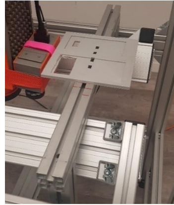
Figure 3.14: 3D-printed smartphone bracket over hyperspectral imaging system.
