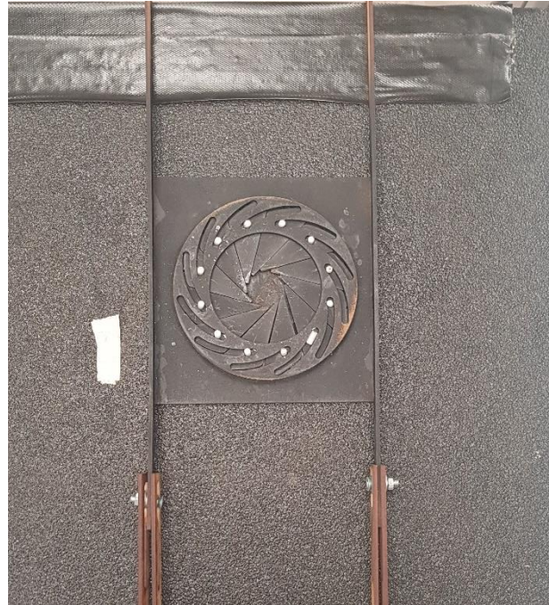
Figure 3.4: Iris Mechanism used to Kiwifruit during hyperspectral image capture.
