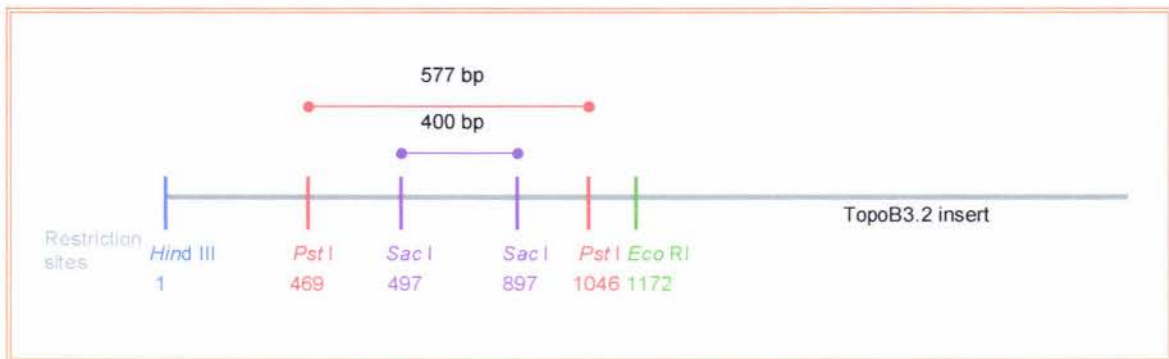
Figure 3.9: Schematic representation of restriction sites within TopoB3.2 insert. Theoretical restriction sites (coloured lines) within TopoB3.2corrected were estimated using the Map program within GCG (Version 9.1; Wisconsin Genetics Computer Group, USA). The Hind III restriction site represents the T3 primer side of the MCS within pBluescript SK (+). Each restriction site would generate fragments of identical sizes to those observed in the actual restriction digests (section 3.3.1, appendix 3.1).
