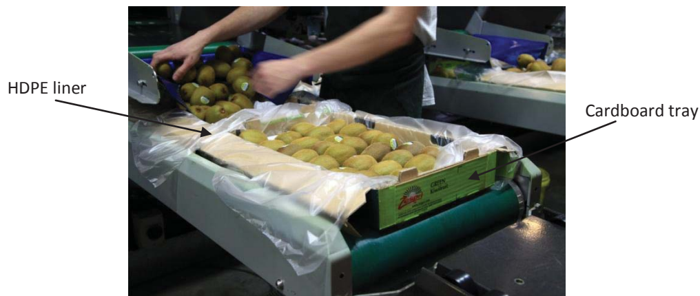
Figure 3.2: Kiwifruits packed in single layer in cardboard tray and covered with HDPE liner.
