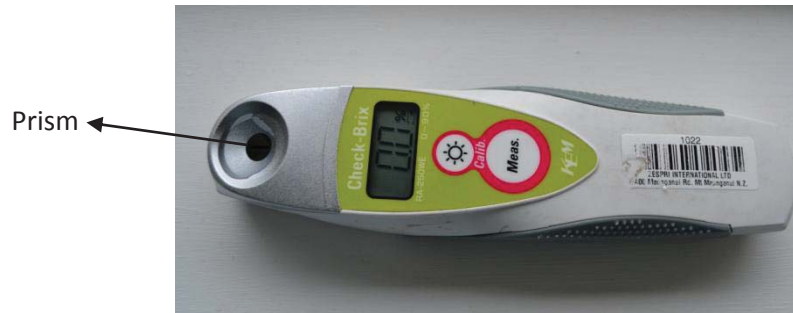
Figure 3.14: Refractometer (RA-250WE, KEM, Japan) calibrated to ‘zero’ before measurement of SSC in kiwifruit
