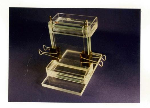
Gel drying apparatus. The gels were dried to prepare permanent (non-photographic) records and for fluorography. This system was composed of:
