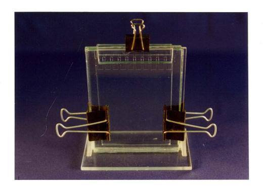
Assembly of the gel apparatus. The glass plates were removed from the gel pouring stand. The bottom perspex spacer was removed and the plates clamp on to the electrophoresis stand. "Threads" of petroleum jelly were placed around the notched glass plate to stop leakage or short circuits.
