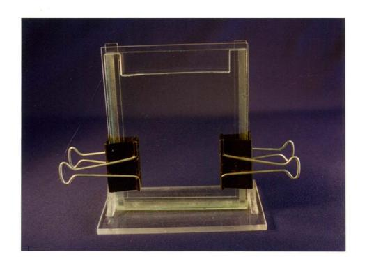
Pouring the gel. Unpolymerised acrylamide was poured between the two glass plates (positioned at approximately 45° to the vertical) until the desired column length (110 mm) of acrylamide was reached. The plates were positioned vertically and a layer, approximately 5 mm high, of distilled water was poured on top of the gel. Note that there is a visible acrylamide/water interface after polymerisation of the gel is complete.
