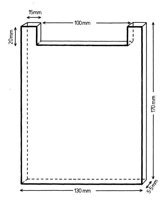
Assembly of the glass plates. A "thread" of petroleum jelly was placed around the side and lower edges of one of the glass plates and the perspex spacers were pressed on to the threads. A second "thread" was positioned on to the spacers and the notched glass plate was pressed into position. The glass "sandwich" was clamped to the stand and was then ready for the pouring of the unpolymerised gel solution.
