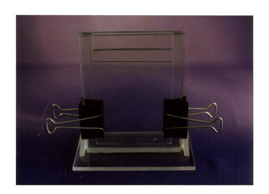
Preparation of gradient gels. Solutions of two different acrylamide concentrations are placed in the conical reservoirs. The higher acrylamide concentration is next to the peristaltic pump and the valve is opened. When pumping begins a stream of air is used to mix the two concentrations as they are drawn from the reservoirs. The mixture is pumped between the two glass plates until the desired gel height is attained.
