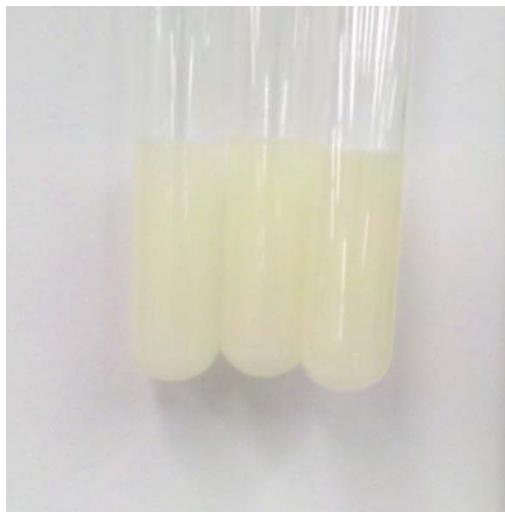
Appendix 4 - Alkaline Phosphatase reaction in UHT milk (A), raw milk (B) and raw milk pasteurised in this study (C).
