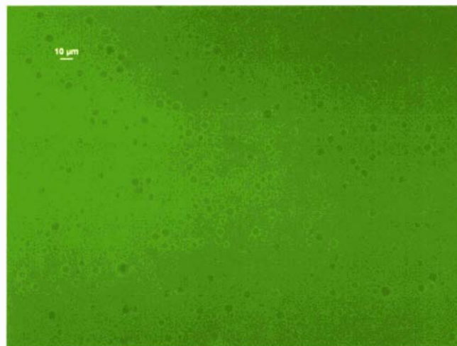
Figure 5.9 Fluorescence image of WGA488-stained fat globules upon adding washed cream to WGA488 stock and reducing the microscope camera exposure time from 148 ms to 6 ms.
