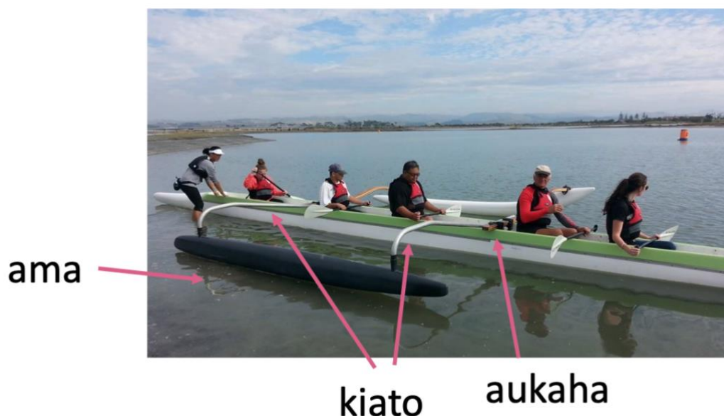
Figure 5: Waka stabilising components. Source: R Nuku, 2015.
