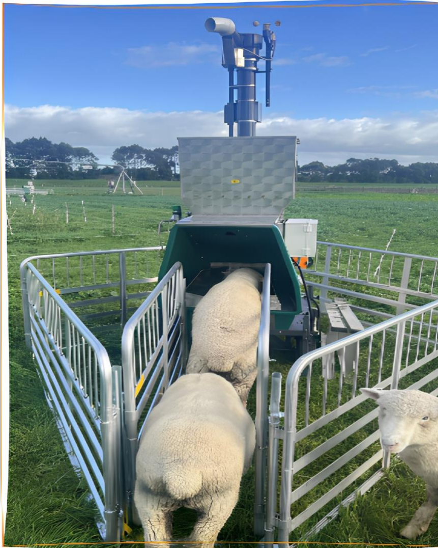
Figure 2.6 GreenFeed system showing sheep voluntarily entering the sampling hood for methane breath measurements under pasture conditions.
