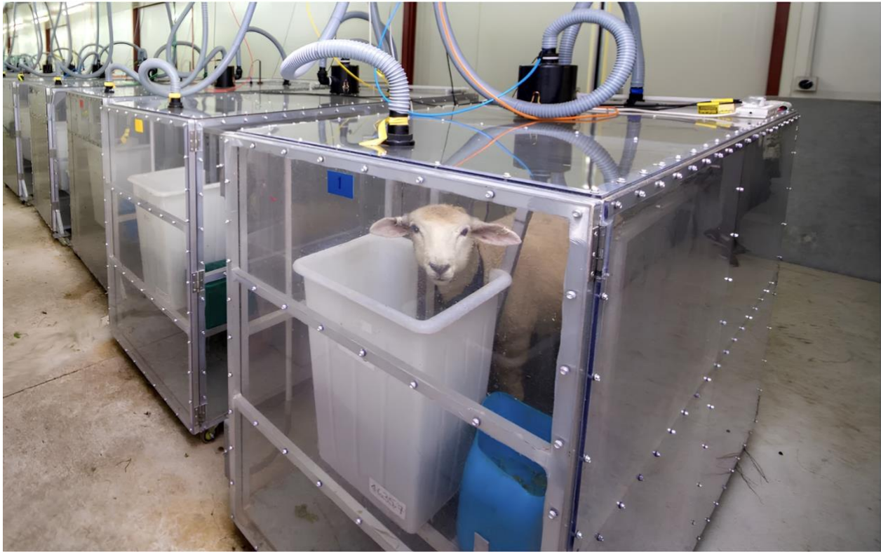
Figure 2.5 Respiration chambers used for measuring enteric methane emissions in sheep at AgResearch, New Zealand.
