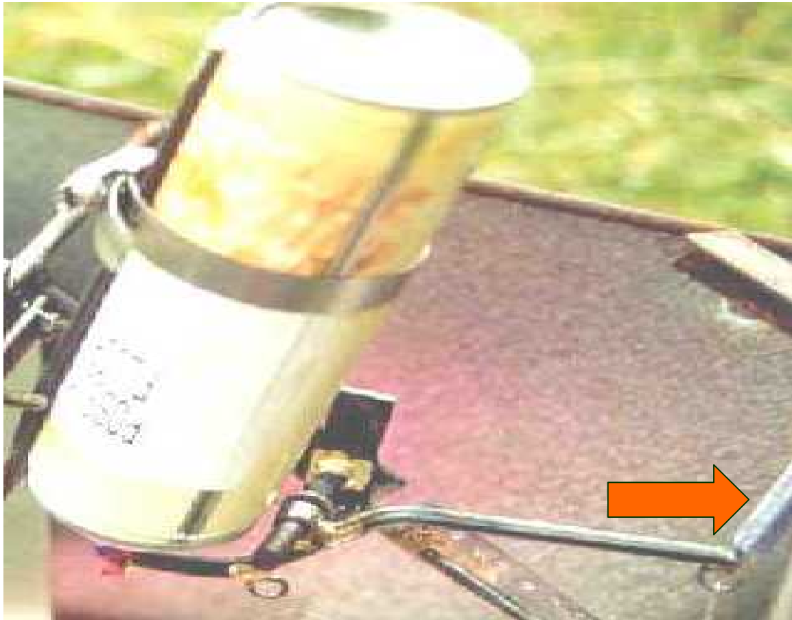
Figure 23. Trigger mechanism and spring (arrowed) on Type three MkII vaccinator
