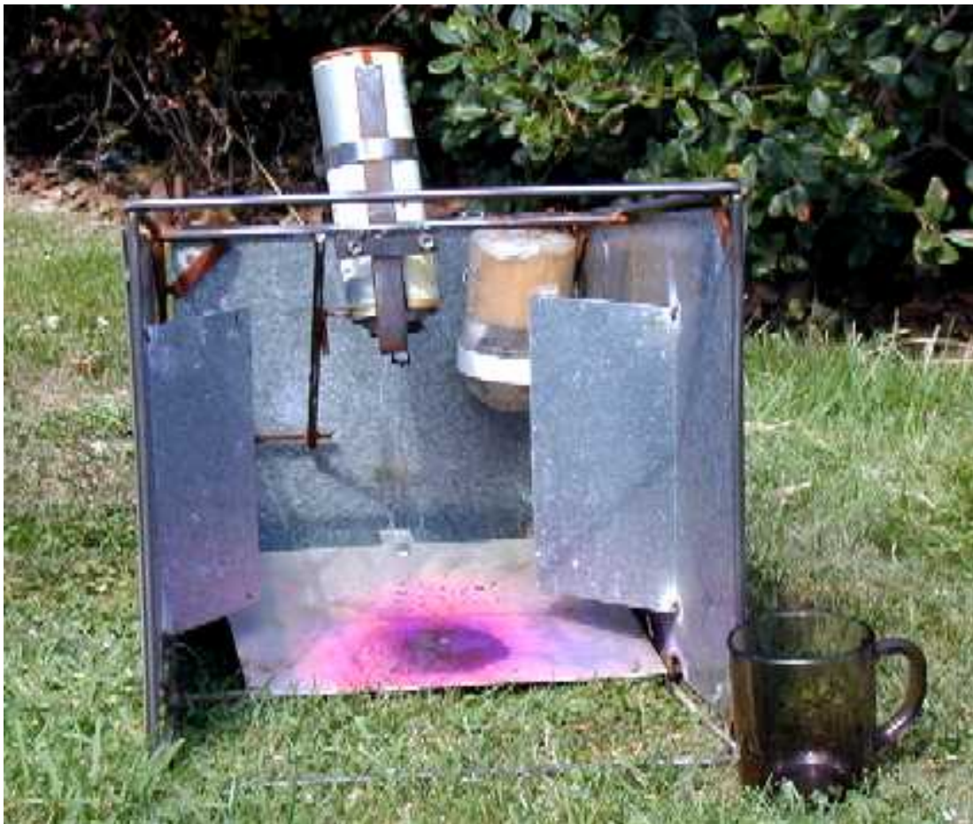
Figure 27. One of twelve steel copies (type 3, Mk VII) of the final vaccinator design after the changes listed in section 4.4.13
