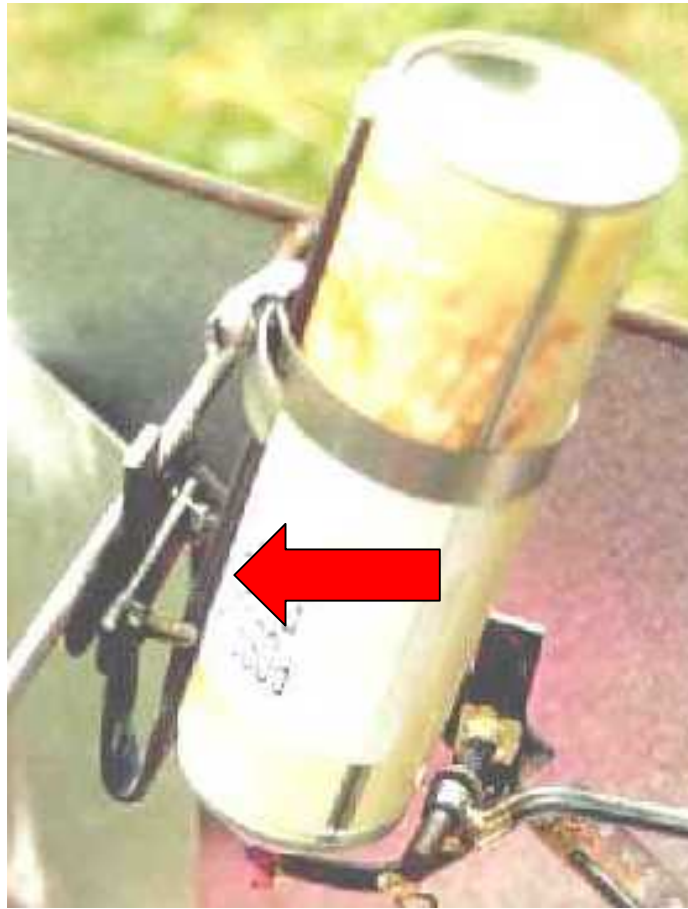
Figure 24. Can holding mechanism showing V shaped steel plate and clamp (arrowed)
