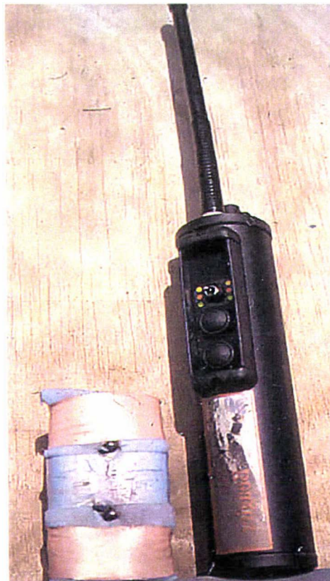
Figure 2.5 “The Beagler” from Tritronics. Three channel remote dog-training device. Electrode on left was attached to the antler
