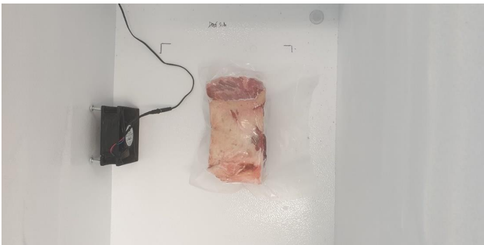
Figure 5: Portable fan installed inside chest freezer for fast freezing experiments
