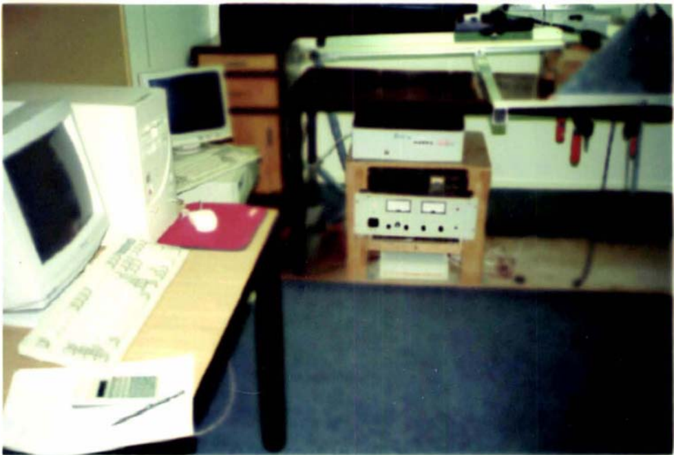
Figure 2.15: (left to right) PC2, PC1, stepping motor (between table legs, near the floor), control box, power supplies and V-scope microprocessor.
