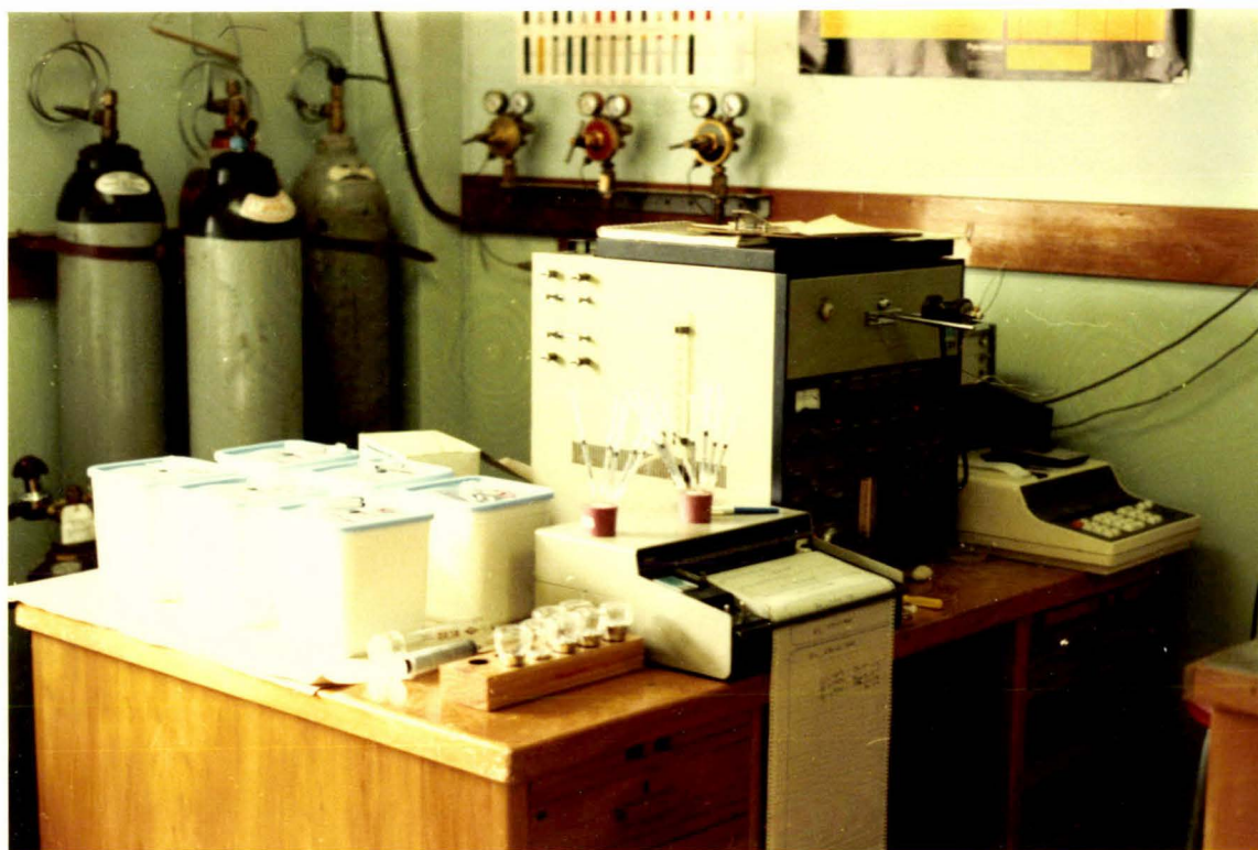
Plate 2 Acetylene reduction technique in progress, showing incubation containers, gas chromatograph and samples awaiting analysis.
