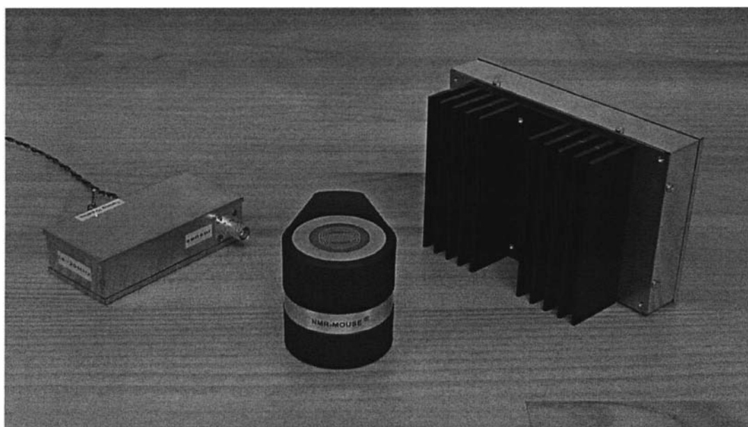
Figure 6.7 NMR-MOUSE with RF front end [22].
