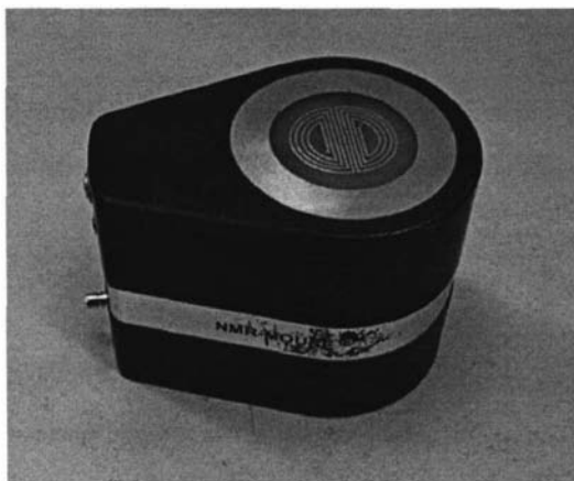
Figure 3.12 The single bar magnet NMR-MOUSE [42]. This probe typically resonates at 19.2 MHz, uses an excitation power level of 100 Watts, has a 90^\circ pulse time of 4 \mu\text{s} and produces a Spin Echo signal with amplitude 10 \mu\text{V} and duration 10 \mu\text{s} .
