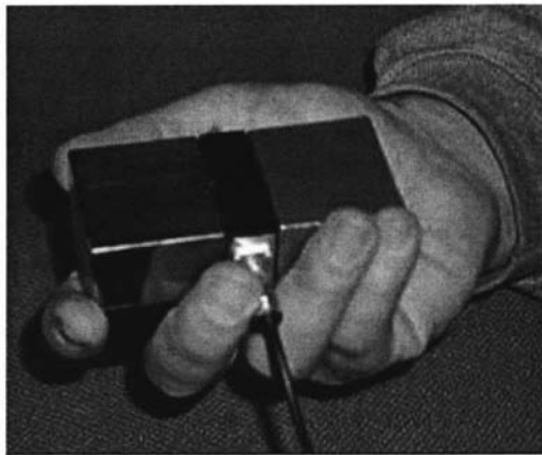
Figure 6. Two magnet, handheld NMR-MOUSE.
