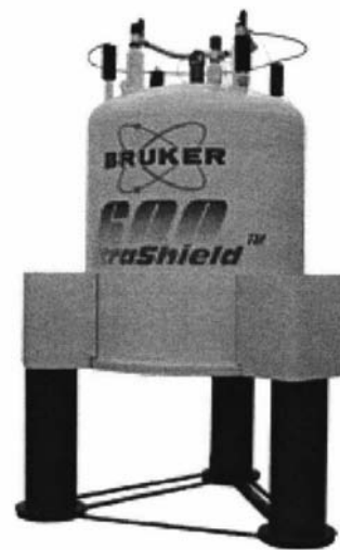
Figure 4. A 14 Tesla superconducting magnet of height approximately 2 m [5].
