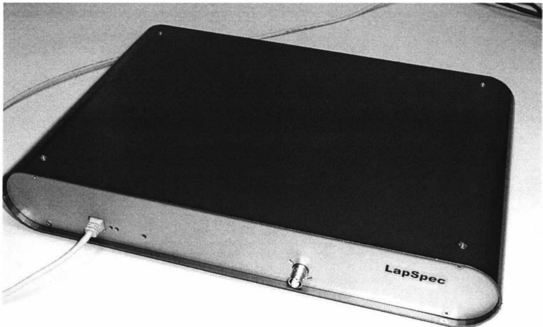
Figure 7.13 Complete Lapspec, measuring 360 x 240 x 55 mm and weighing 3.6 kg.
