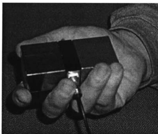
Figure 3.11 Two magnet, handheld NMR-MOUSE. Figure taken from reference 50.
