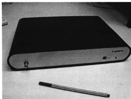
Figure 14. Complete portable NMR spectrometer.
