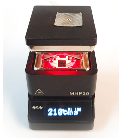
Figure 3.14: MHP30 mini hot plate with conductive fabric test square.
