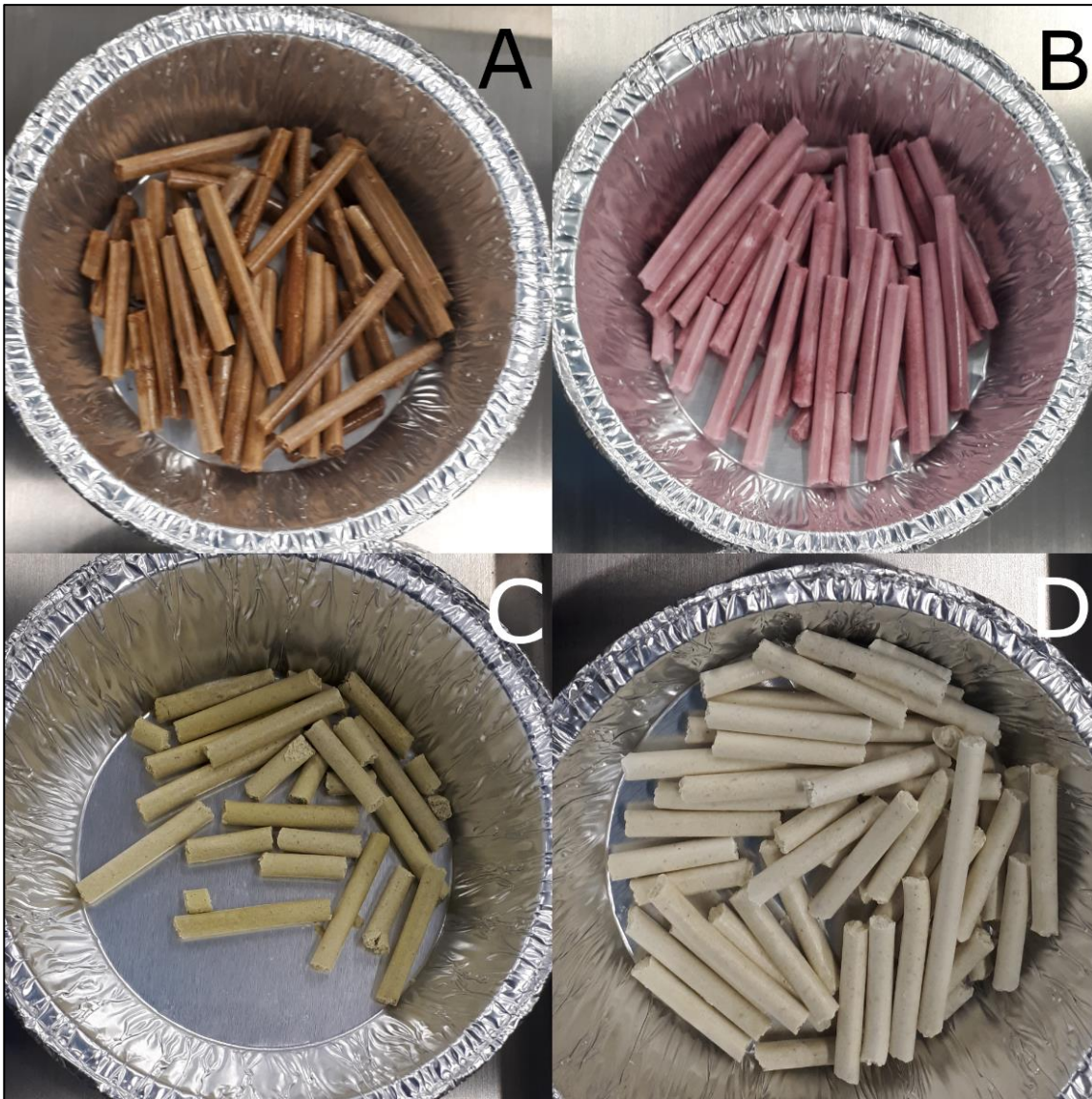
Figure 7-13: Samples of product that was vacuum freeze-dried after rapid freezing and extrusion. A: 20.4° Brix coffee extract. B-D: Fruit smoothie mixes.
