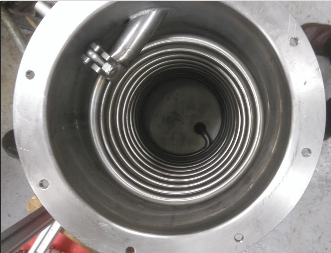
Figure 7-4: Spiral Freezer tube, showing the spiral construction and the exterior of the coolant annulus. The plug that forms the annulus is not shown.
