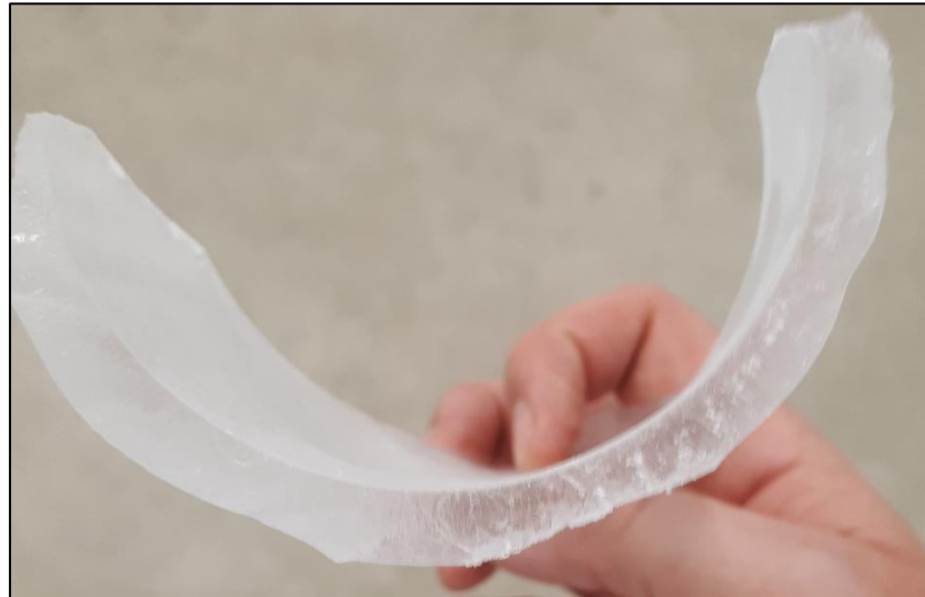
Figure 3-27: Ice flake of approximately 10mm thickness detached by rapid heating of the internal tube surface.
