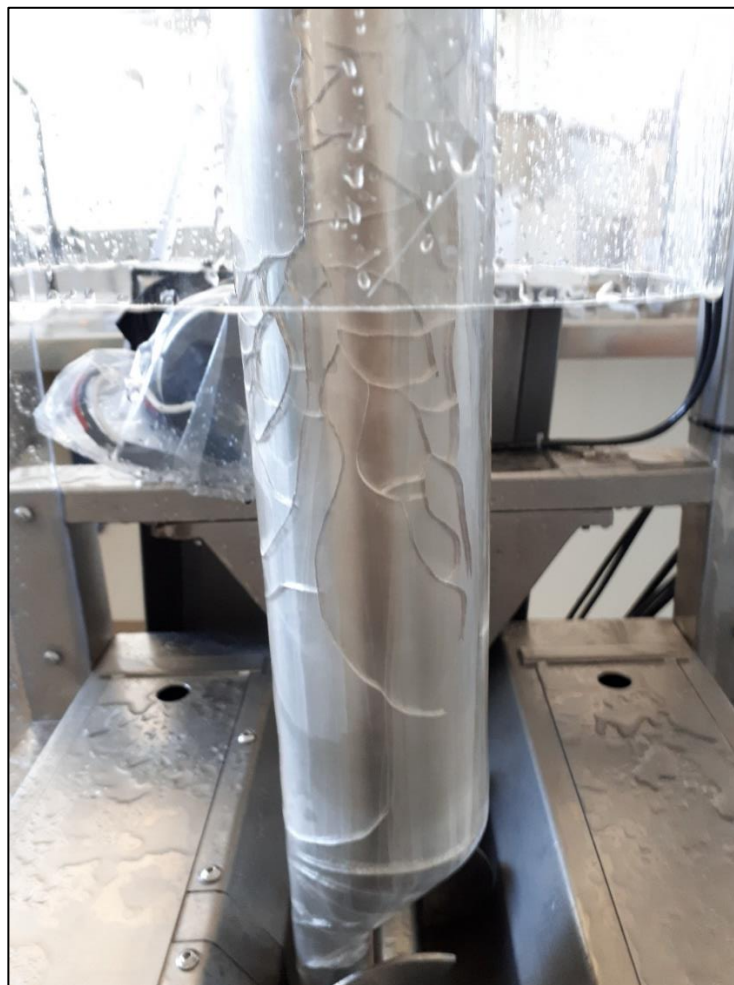
Figure 3-28: Cracking of water ice layer (approx. 5mm thickness) during rapid heating of internal surface of freezer tube.
