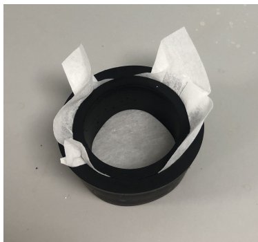
Figure 7.1: Filter holder setup for nematode extraction.
