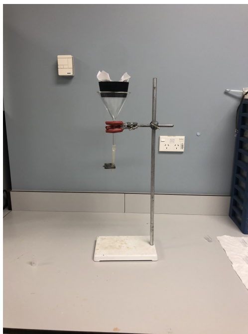
Figure 7.2: Baermann funnel setup for extracting nematodes.
