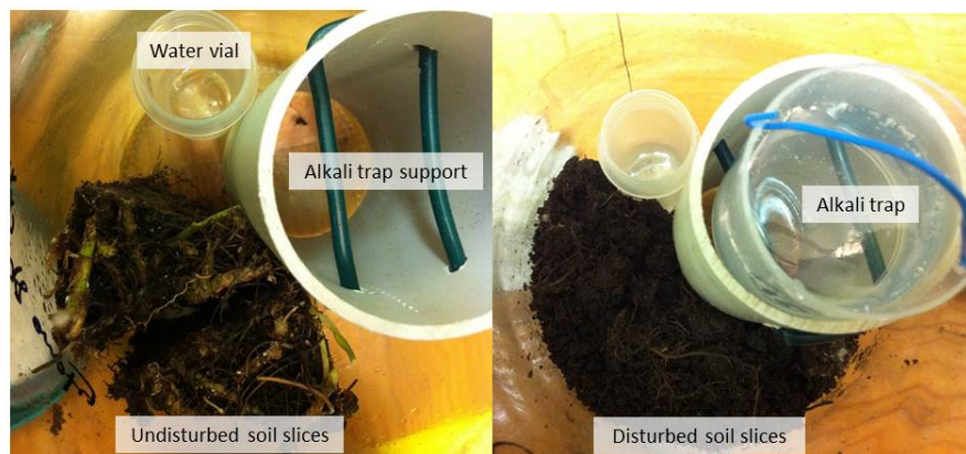
Figure 4.5 Ready for incubation: intact (undisturbed) soil slices (left); chopped and sieved (disturbed) soil slices (right).
