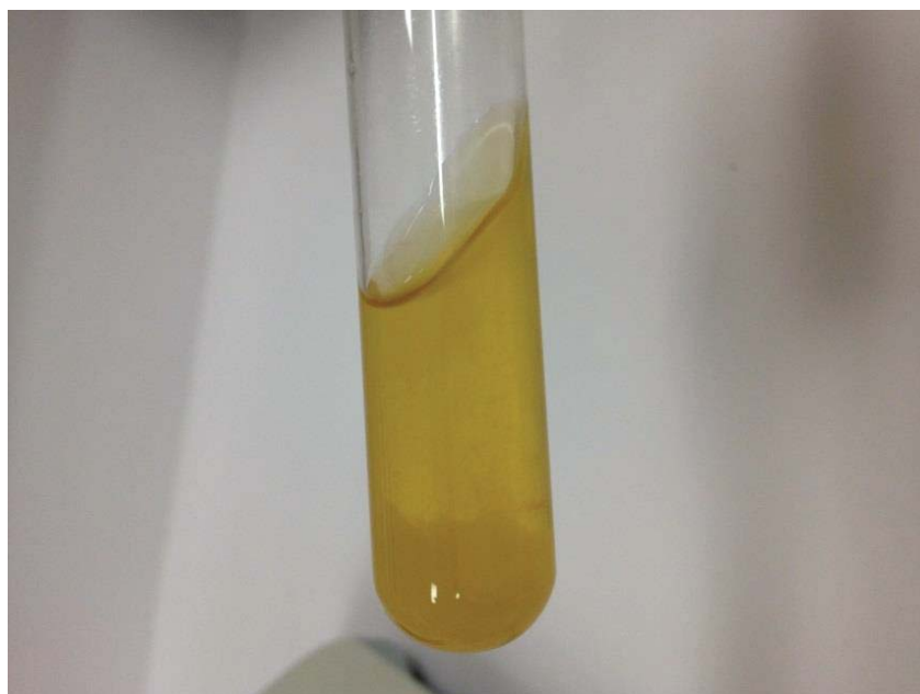
Figure D2 An example of coagulate-positive result of one counted colony from a Petrifilm.
