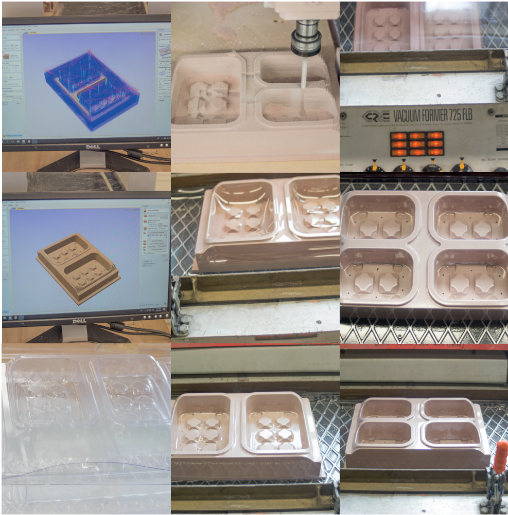
Figure 58: Creation of moulds and thermo-foming process
