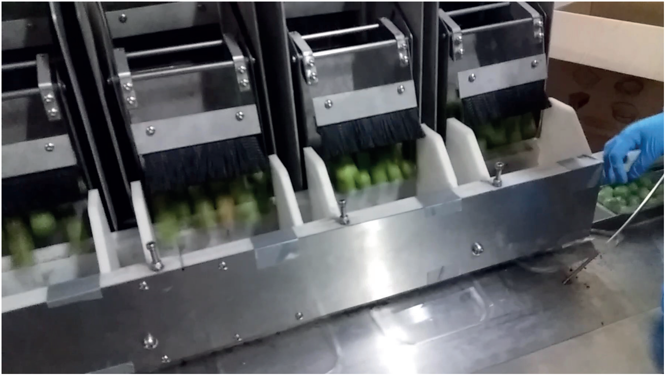
Figure 15: Kiwiberries being loaded into clamshells and manually shaken to settle the berries
