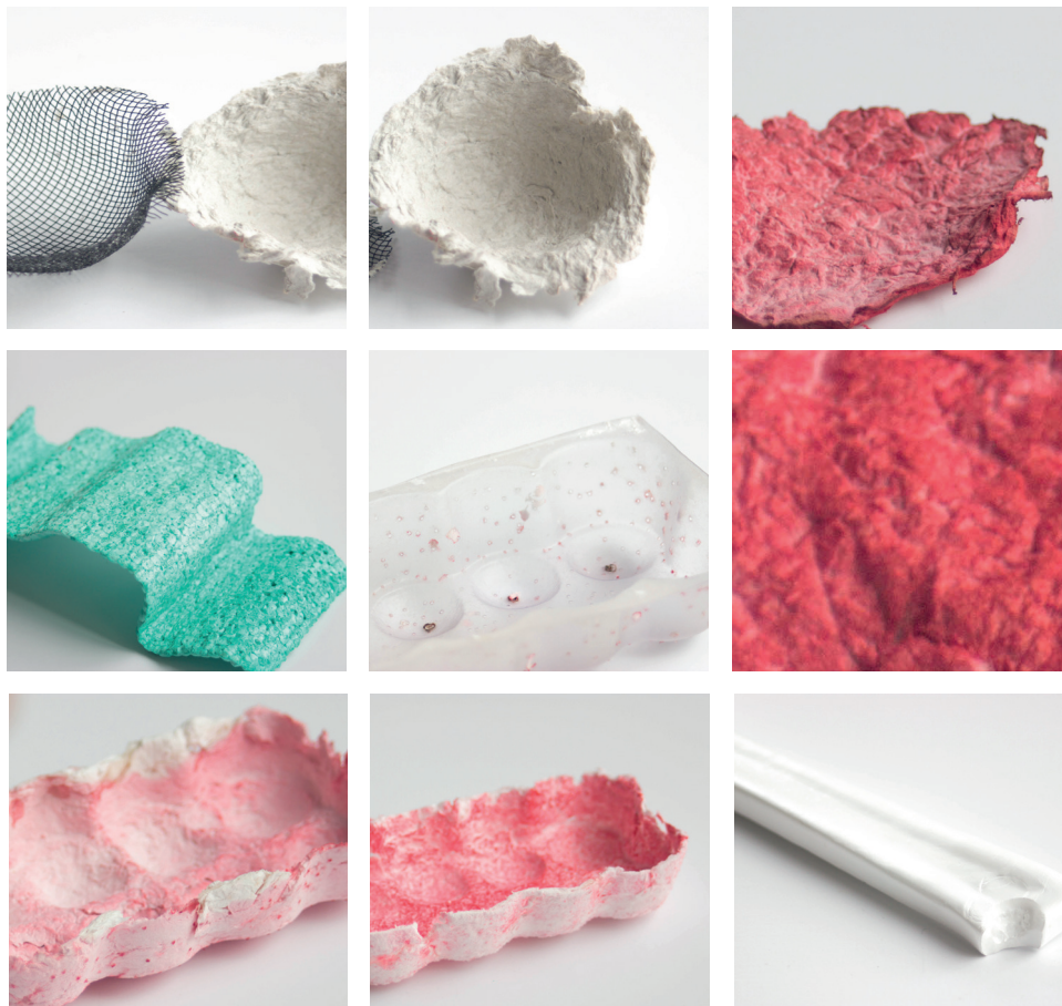
Figure 27: Material explorations with moulded fibre, PLA foam and thermo-formed plastics
