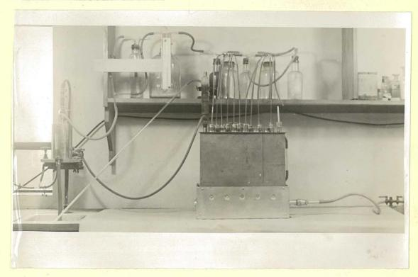
Shows "Swfit Stability Tester" for testing oxidation of ghee samples by accelerated test at 100°C.
