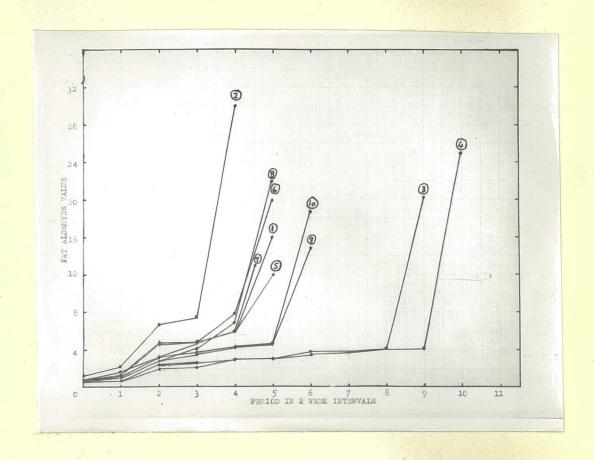
Fig. 9. Graph showing oxidation and induction periods
