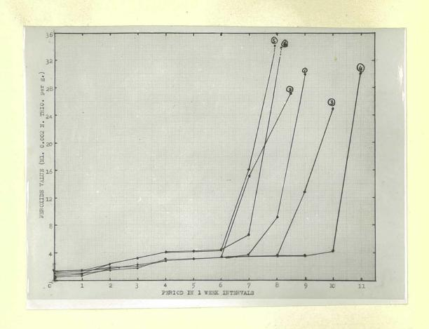
Fig. 5. Graph showing oxidation and induction periods by Peroxide method (details given in Table 4, page 31).
