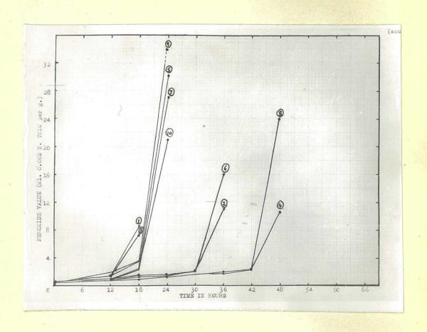
Fig. 18. Graph showing oxidation and induction periods by accelerated test at 100°C. (Details given in Table 7, page 50).
