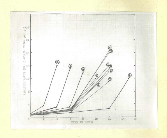
Fig. 26. Graph showing oxidation and induction periods by accelerated test at 100°C. (Details given in Table 12, page 75).
