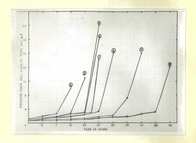
Fig. 20. Graph showing oxidation and induction periods by accelerated test at 100°C. (Details given in table 9, page 60).
