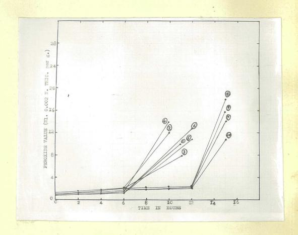
Fig. 27. Graph showing oxidation and induction periods by accelerated test at 100°C. (Details given in Table 14, page 80).
