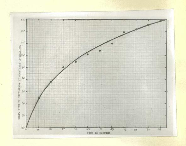
Fig. 22. Graph showing rate (time and temperature) of slow heating.
