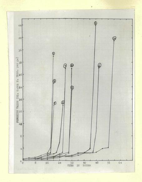
Fig. 14. Graph showing oxidation and induction periods by accelerated test at 100°C. (Curves 1 - 6 correspond with treatments listed in Table 6, page 43).
