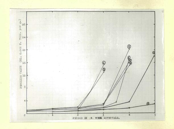
Fig. 19. Graph showing oxidation and induction periods by peroxide method. (Details given in Table 9, page 60).
