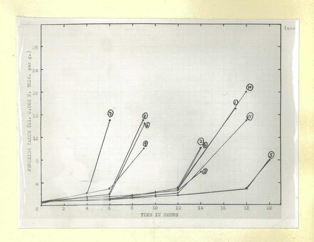
Fig. 25. Graph showing oxidation and induction period by accelerated test at 100°C. (Details given in Table 11, page 72).
