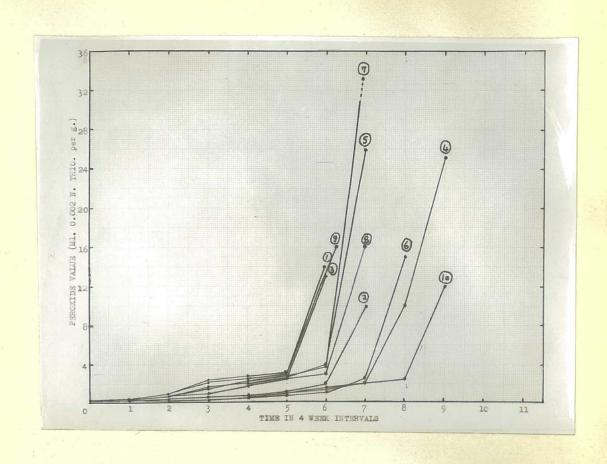
Fig. 11. Graphs showing oxidation and induction periods by Peroxide method. (Details given in Table 6, page 43).
