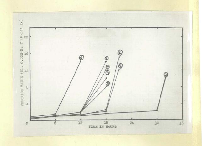
Fig. 24. Graph showing oxidation and induction periods by accelerated test at 100°C. (Details given in Table 10, page 66).
