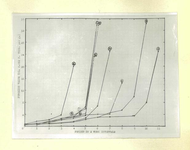
Fig. 8. Graph showing oxidation and induction periods by Peroxide method (details given in Table 5, page 37).
