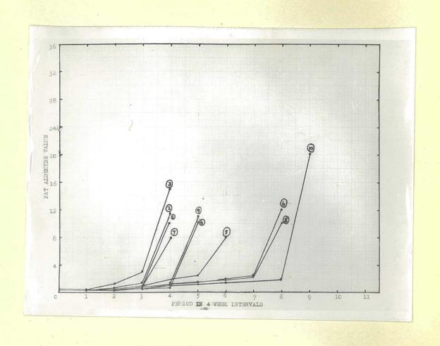
Fig. 16. Graph showing oxidation and induction period by fat aldehyde method. (Curves 1 - 6 correspond with treatments listed in Table 7, page 50).
