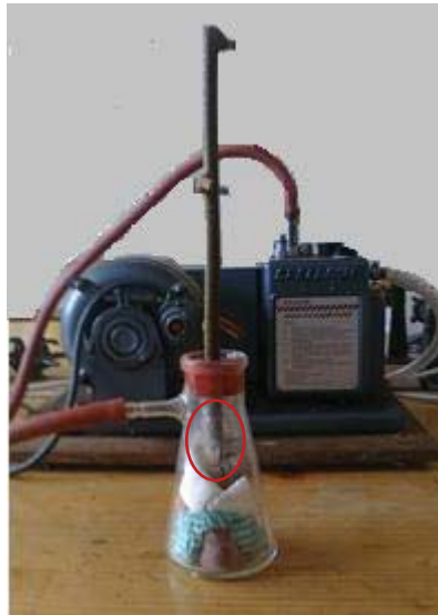
Figure 2.4 Equipment set-up for xylem sap extraction from shoots, illustrating section of a kiwifruit shoot inserted into a vial, held within an airtight Buchner flask (front) connected to a vacuum pump (back) (red circle indicates vial placed in the Buchner flask for collection of fluid).
