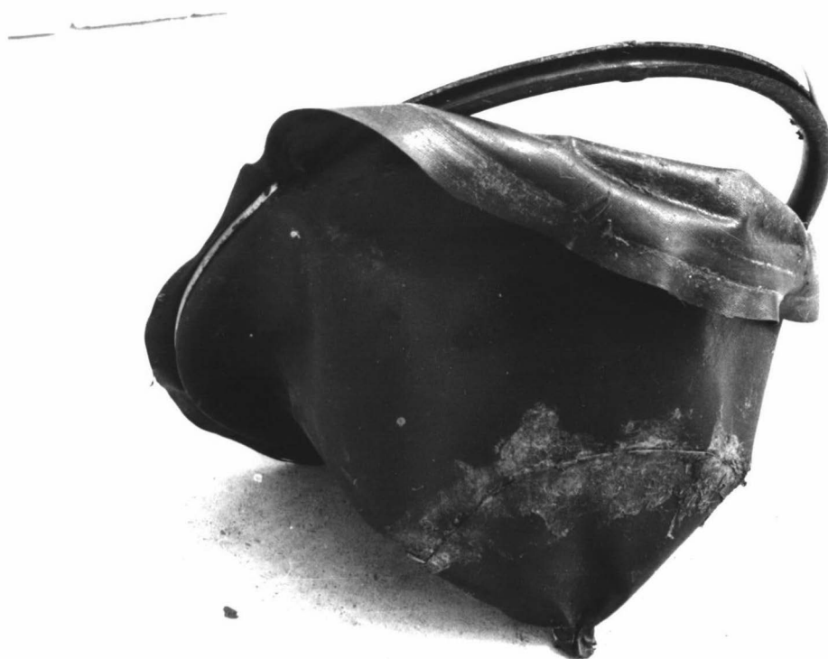
PLATE 2.4 Butyl rubber, urine collection funnel partially dismantled. Note the vacuum strip seal alkathene frame and the totally collapsible rubber funnel.
