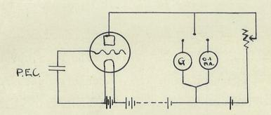
A Phillips A.415 valve was found to give the most stable reading on the galvanometer.
