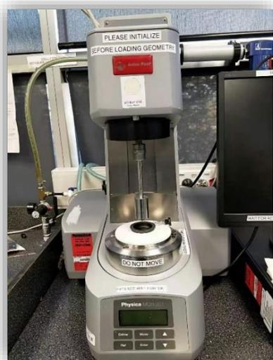
Figure 3-1 Rheometer MCR 301
