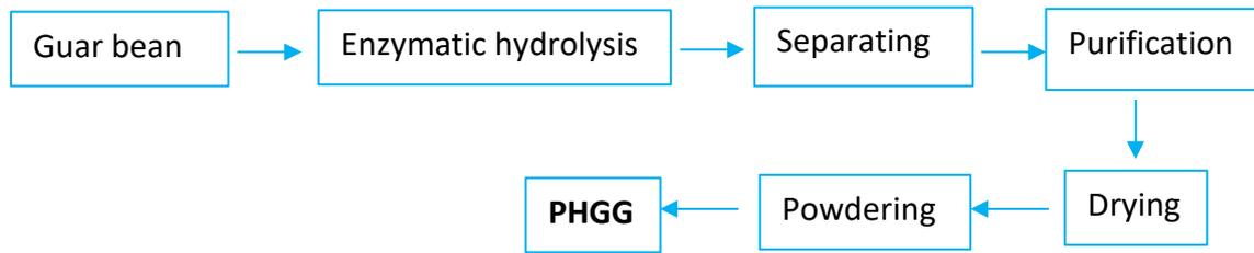
Figure 2-4 The processing of PHGG
