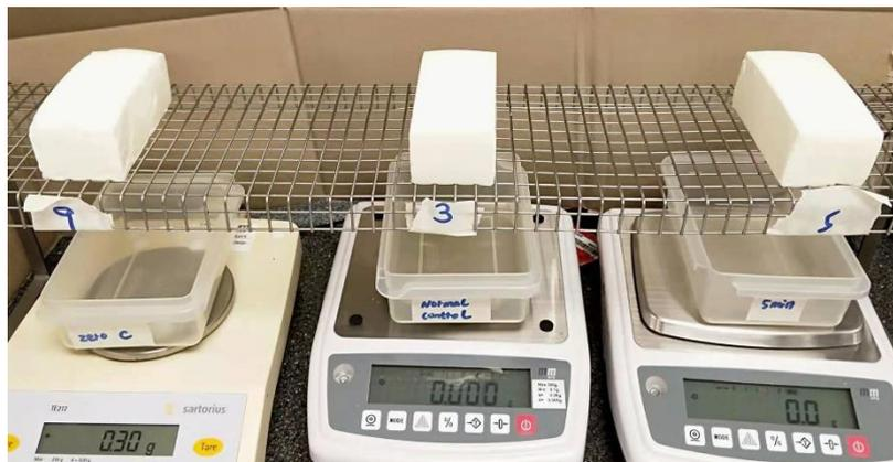
Figure 3-4 Measurement of ice cream melt down rate
