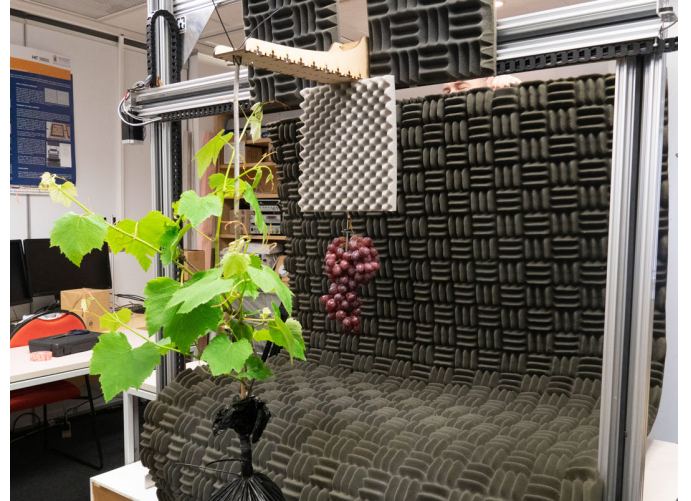
(a) A small vine was positioned in front of a cluster of grapes supported by a custom laser cut gantry tower fixed to a vertically orientated CNC machine. Acoustic damping foam was employed to reduce acoustic reflections from aluminium CNC components and reduce reverberations throughout the room.
