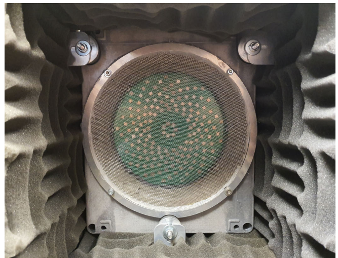
Fig. 1: View of the ultrasonic arrays main PCB installed in the measurement unit. The transducers can be seen in gold, arranged in an optimised spiral pattern.
