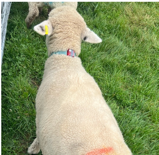
Figure 3.3 ActiGraph ® accelerometer attached to the collar and placed ventrally on the neck of the ewe lamb.
