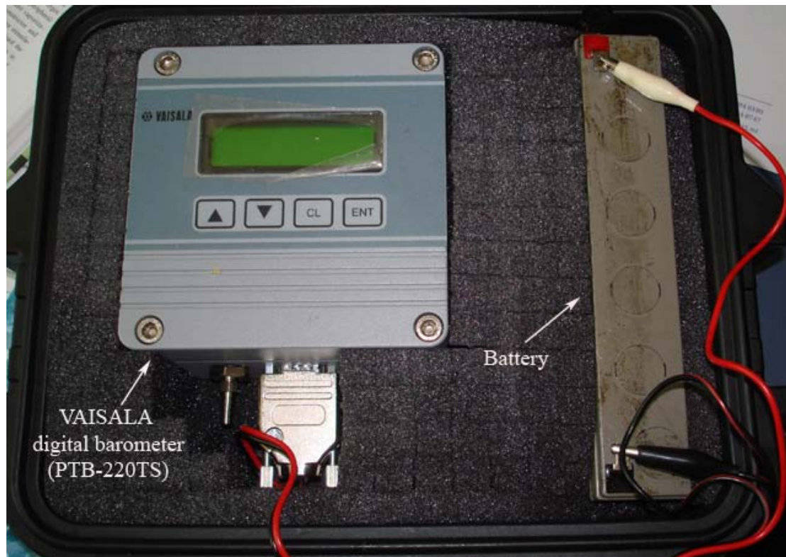
Figure 2.4.1 The reference barometer (VAISALA digital barometer [PTB-220TS]) and battery. The barometer and battery is fitted in a portable box.
