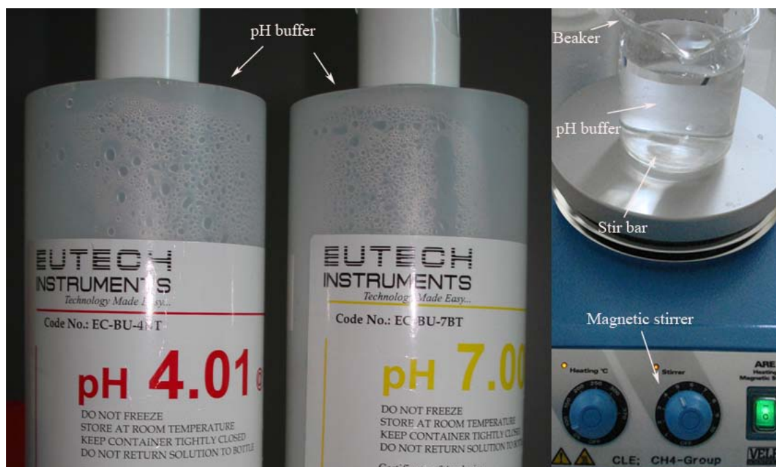
Figure 2.5.1 Equipments used for pH calibration: pH 4.01 buffer solution, pH 7.00 pH buffer solution, beaker, magnetic stirrer and stir bar.
