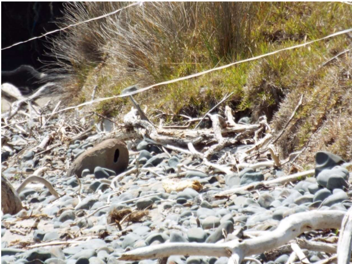
Plate 2.6 Camera enclosed in artificial rock deployed near the entrance of a tūturuatu nest.
