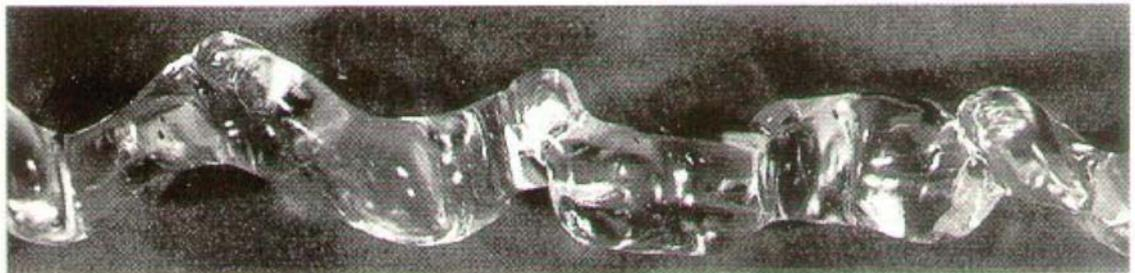
**Figure 2.14** Melt fracture or gross distortion of extrudate passing through a die well above its critical stress (Black, 2000).
