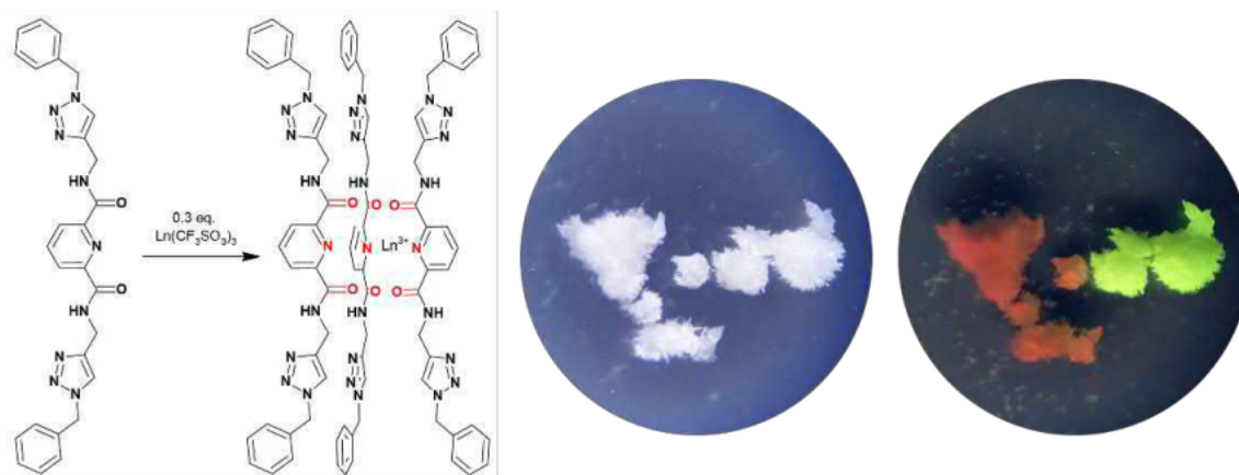
Figure 3.1. (Left) Ligand 2 coordinating to \text{Ln}^{3+} to form a 1:3 metal:ligand species. (Right) Solid \text{Eu}(\mathbf{2})_3(\text{CF}_3\text{SO}_3)_3 and \text{Tb}(\mathbf{2})_3(\text{CF}_3\text{SO}_3)_3 crystalline complexes under a microscope, firstly under ambient light and then under shortwave UV irradiation ( \lambda_{\text{exc}} = 254 \text{ nm} ).
