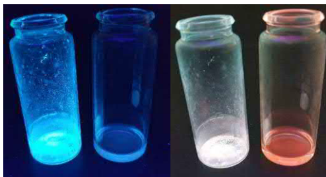
Figure 5.63. \text{Eu}(\mathbf{6})_3 solid and 0.01 mM MeCN solution under longwave irradiation (Left, \lambda_{\text{ex}} = 254 nm) and shortwave irradiation (Right, \lambda_{\text{ex}} = 365 nm).
