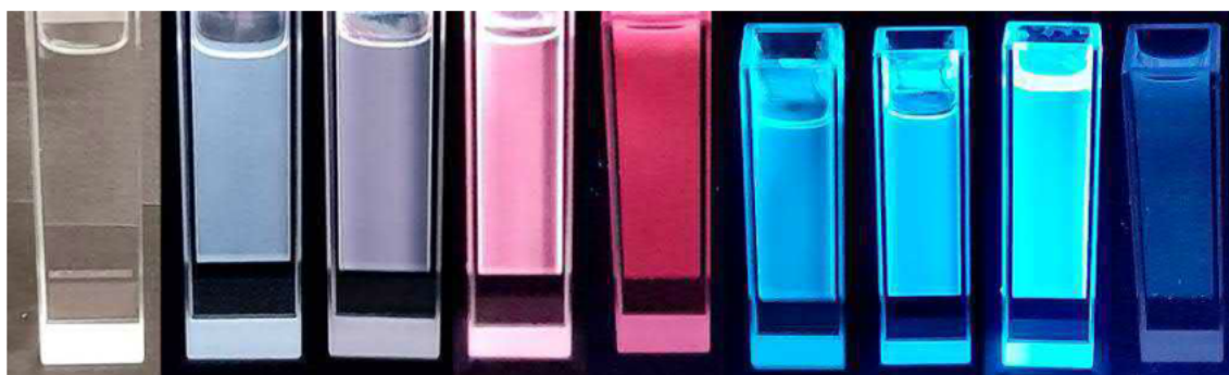
Figure 5.66. \text{Eu}(\mathbf{6})_3 in MeOH solutions with 10, 5, 1, 0.01 mM concentrations left to right, under shortwave UV irradiation (white and red) and under longwave UV irradiation (blue).
