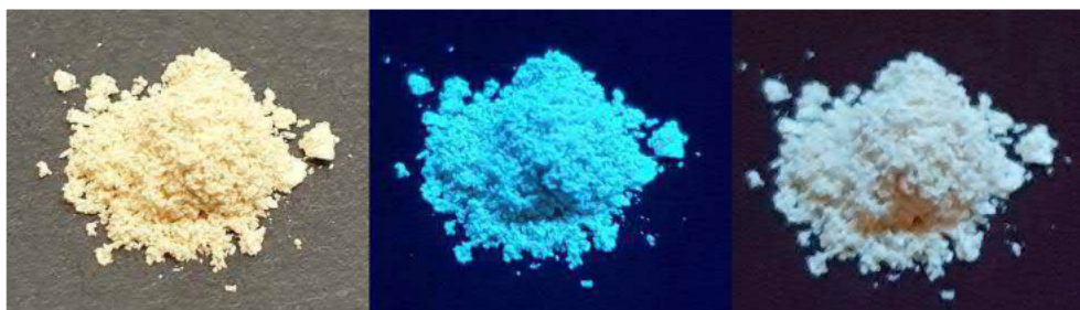
Figure 5.72. Solid powder of \text{Eu}(\mathbf{8})_3 under ambient light, longwave irradiation ( \lambda_{\text{ex}} = 365 nm), and shortwave irradiation ( \lambda_{\text{ex}} = 254 nm), from left to right.
