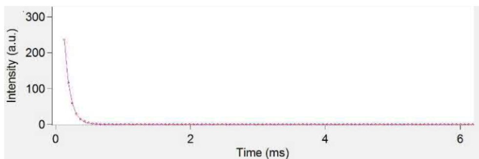
Figure 8.1.59. Lifetime measurement and single exponential fit for [\text{Tb}(3)_3](\text{CF}_3\text{SO}_3)_3 (0.01 mM, MeCN, \lambda_{\text{ex}} = 274\text{nm} , measured at 545 nm)...
