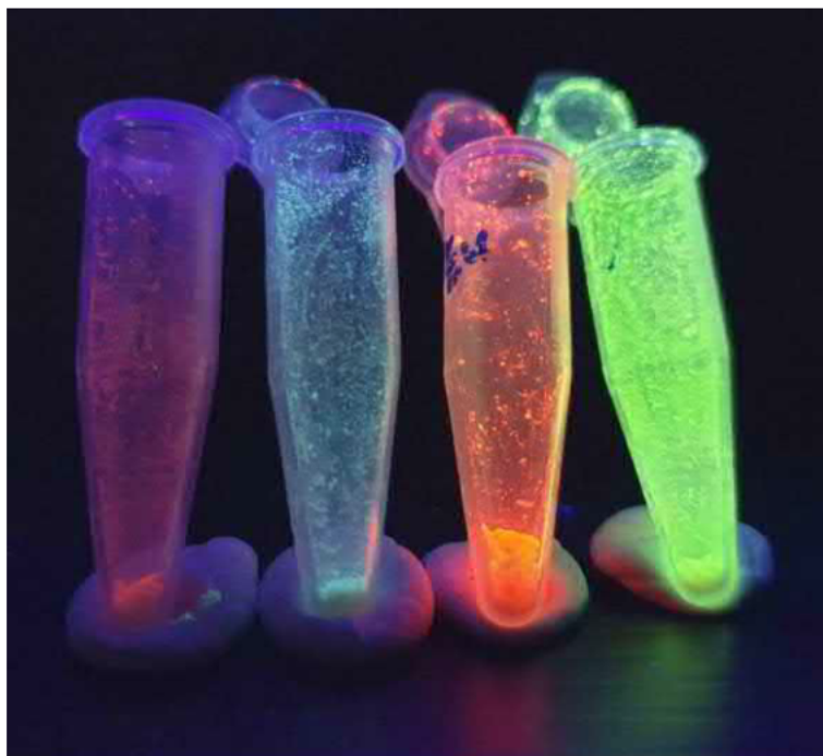
Figure 4.35. Lanthanide complexes Ln( 5 ) 3 under shortwave UV irradiation ( \lambda_{\text{ex}} = 254 \text{ nm} ): left to right - Sm( 5 ) 3 , Dy( 5 ) 3 , Eu( 5 ) 3 and Tb( 5 ) 3
