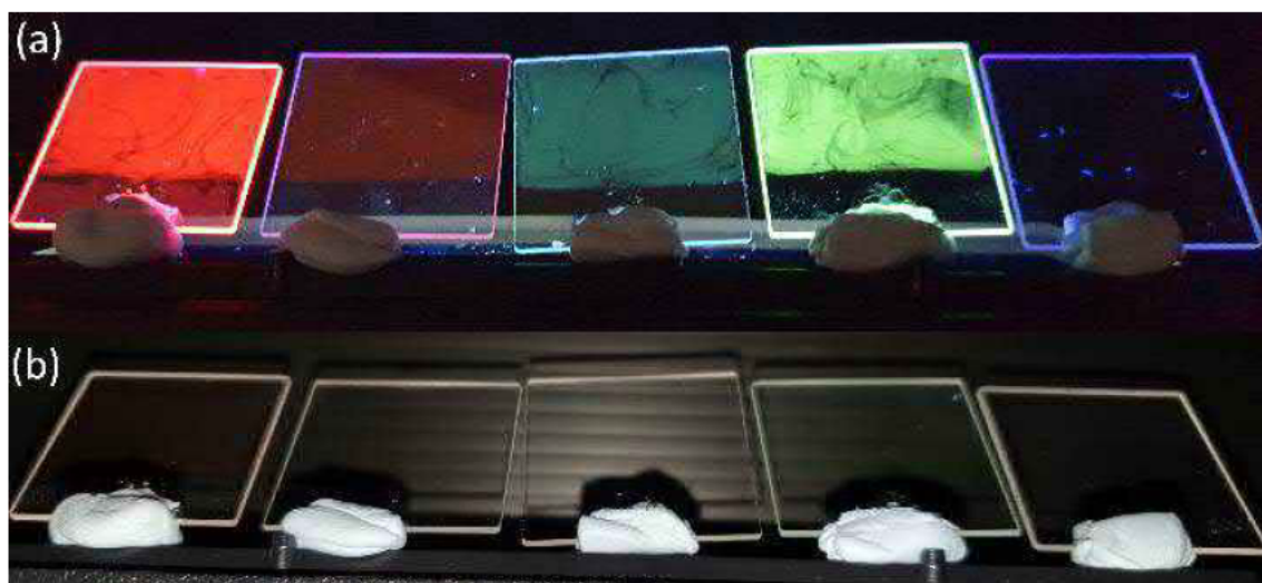
Figure 4.39. LB films of \text{Ln}(\mathbf{5})_3 , (where \text{Ln} = \text{Eu}^{3+} , \text{Tb}^{3+} , \text{Dy}^{3+} and \text{Sm}^{3+} ) shown under shortwave UV irradiation. (a), \lambda_{\text{ex}} = 254 \text{ nm} ) and ambient light. (b). From left to right LB films are \text{Eu}(\mathbf{5})_3 , \text{Sm}(\mathbf{5})_3 , \text{Dy}(\mathbf{5})_3 , \text{Tb}(\mathbf{5})_3 , and a blank slide.
