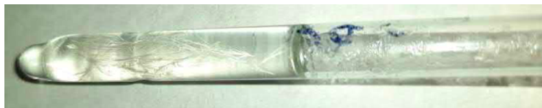
Figure 4.15. Image of crystals of 5 and pipette reactor from which they were grown in.
