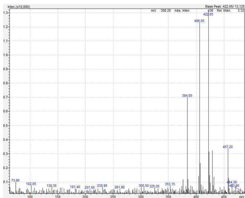
Figure 8.1.8. LRMS m/z = 384.05 . [ 1 + H] ^+ : (calc. for \text{C}_{17}\text{H}_{22}\text{N}_3\text{O}_3^+ , 384.19), m/z = 406.05 . [ 1 + Na] ^+ : (calc. for \text{C}_{17}\text{H}_{21}\text{N}_3\text{O}_2\text{Na}^+ , 406.17) and m/z = 422.05 . [ 1 + K] ^+ : (calc. for \text{C}_{17}\text{H}_{21}\text{N}_3\text{O}_2\text{K}^+ , 422.15)..
