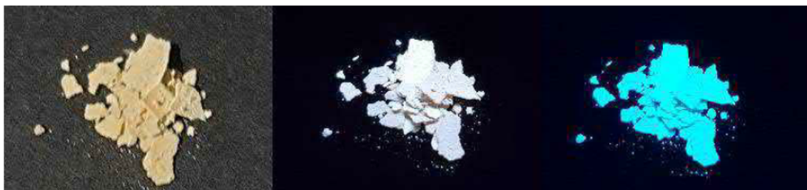
Figure 5.60. \text{Eu}(\mathbf{6})_3 solid powder, under ambient light, shortwave UV irradiation ( \lambda_{\text{ex}} = 254 \text{ nm} ), and longwave UV irradiation ( \lambda_{\text{ex}} = 365 \text{ nm} ), from left to right.
