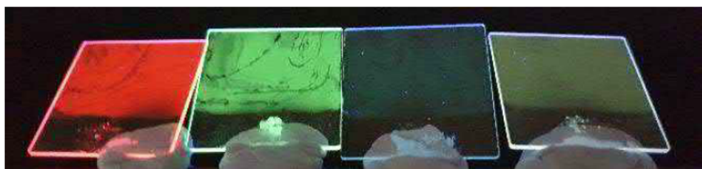
Figure 4.64. Image of three monolayer LB films of \text{Ln}(\mathbf{5})_3 (where \text{Ln}^{3+} = \text{Eu}^{3+}, \text{Tb}^{3+} and \text{Dy}^{3+} , respectively) and the final triple mixed monolayer LB film of \text{Eu}(\mathbf{5})_3:\text{Tb}(\mathbf{5})_3:\text{Dy}(\mathbf{5})_3 (1:1:10) on the right, all under shortwave UV irradiation ( \lambda_{\text{exc}} = 254 \text{ nm} ).
