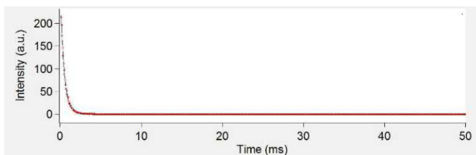
Figure 8.1.31. Lifetime measurement and single exponential fit for [Eu(1)_3](CF_3SO_3)_3 (0.01 mM, MeCN, \lambda_{ex} = 274 nm, measured at 616 nm)...
