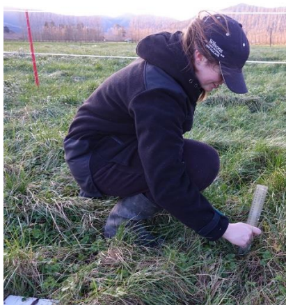
Figure 8: Pre-plot mud-depth measurement being taken.
