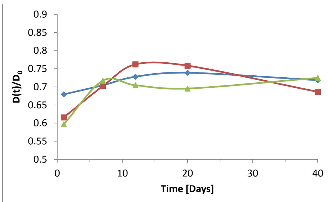
**Figure 10.13: Normalised diffusion of water at 500 ms within the Mozzarella samples over the storage trial at 25°C [◆Low (129), ■Control (148) and ▲High (171)].**
