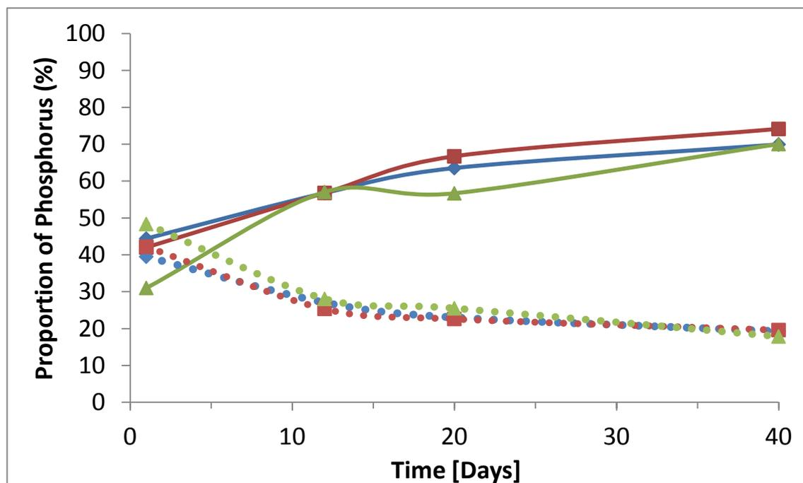
**Figure 10.18: Change in the proportion of mobile phosphorus (solid line) and immobile phosphorus (dashed line) containing groups over the 40 day storage trial [◆Low (129), ■Control (148) and ▲High (171)].**
