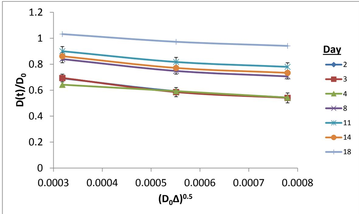
Figure 9.7: Diffusion coefficients of water at 65°C over the storage trial measured using a stimulated echo PGSE sequence in the transverse direction as a function of the observation time. The diffusion coefficients are normalised using the diffusion of free water at 65°C estimated at  $D_0 = 5.00 \times 10^{-9} \text{ m}^2 \text{ s}^{-1}$ .
