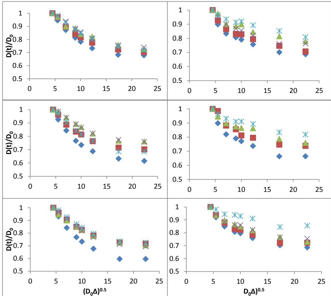
**Figure 10.12: Diffusion of water at 25°C (left) and 65°C (right) for the Mozzarella samples: Low (top), Control (middle) and High (bottom) [◆ Day 1, ■ Day 7, ▲ Day 12, X Day 20 and \* Day 40].**
