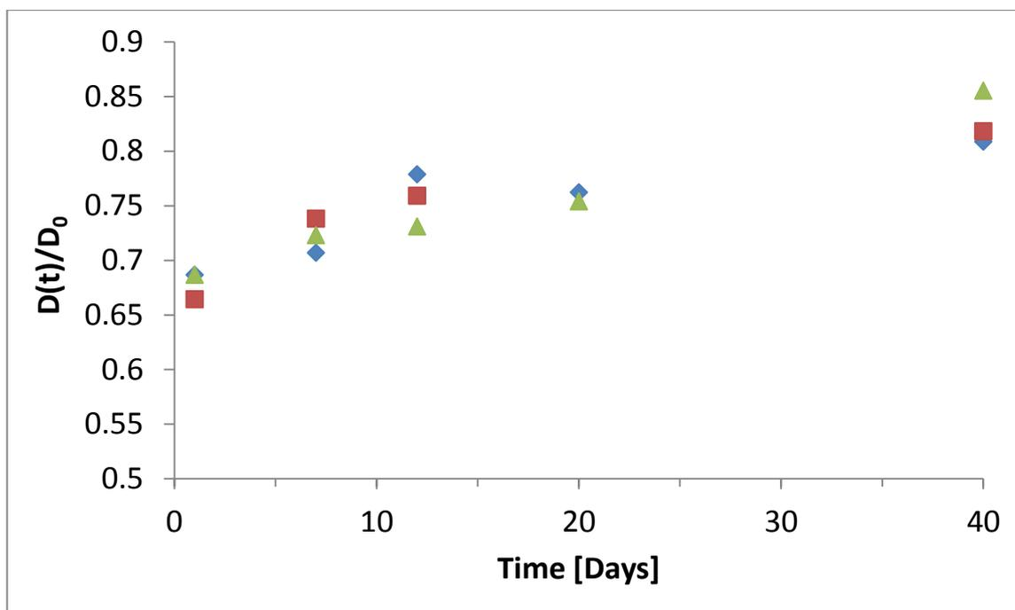
Figure 10.14: Normalised diffusion of water at 500 ms during the storage trial at 65°C [ $\blacklozenge$ Low (129),  $\blacksquare$ Control (148) and  $\blacktriangle$ High (171)].
