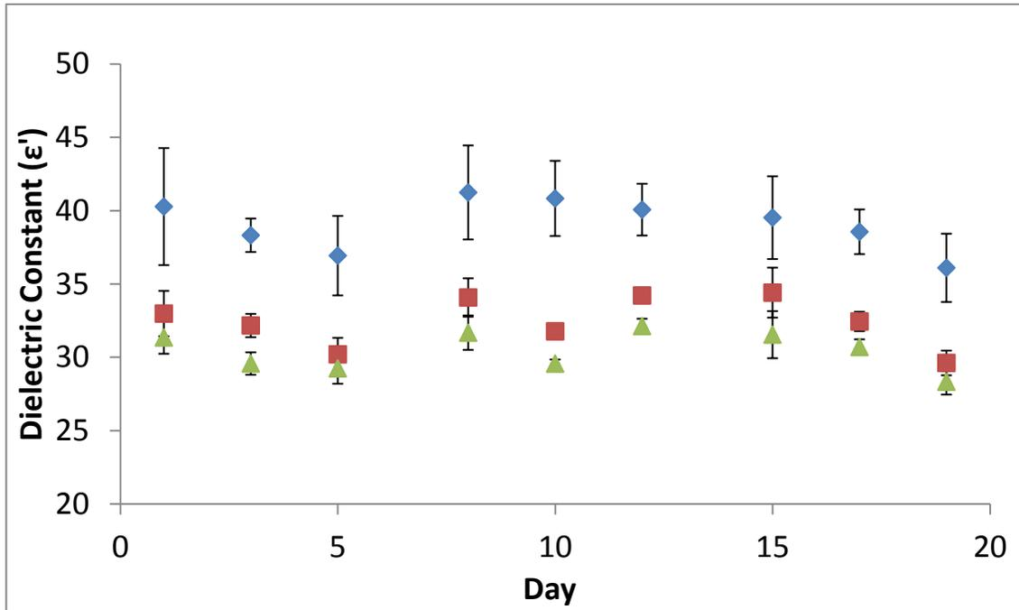
Figure 5.6: Change in the measured dielectric constant over a 20 day period (● 244, ■ 750 & ▲ 1260 MHz)
