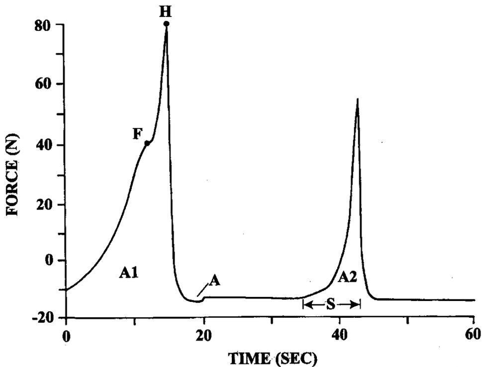
**Figure 2.2: An example of a TPA curve obtained for Mozzarella taken from Tunick (2000).**
