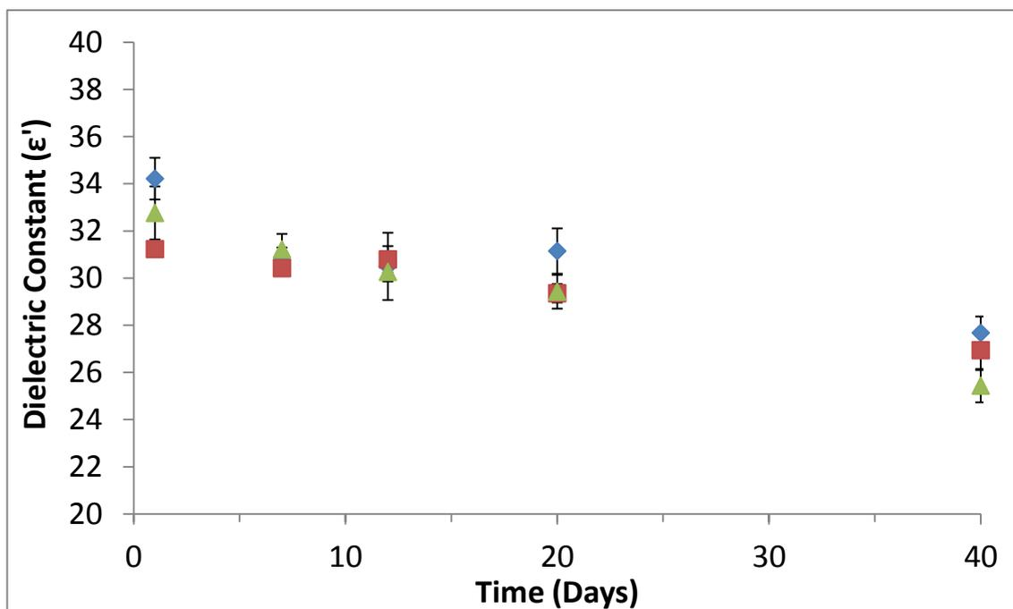
**Figure 10.19: Dielectric constant of the Mozzarella samples over the storage trial at 1.26 GHz [◆Low (129), ■Control (148) and ▲High (171)].**
