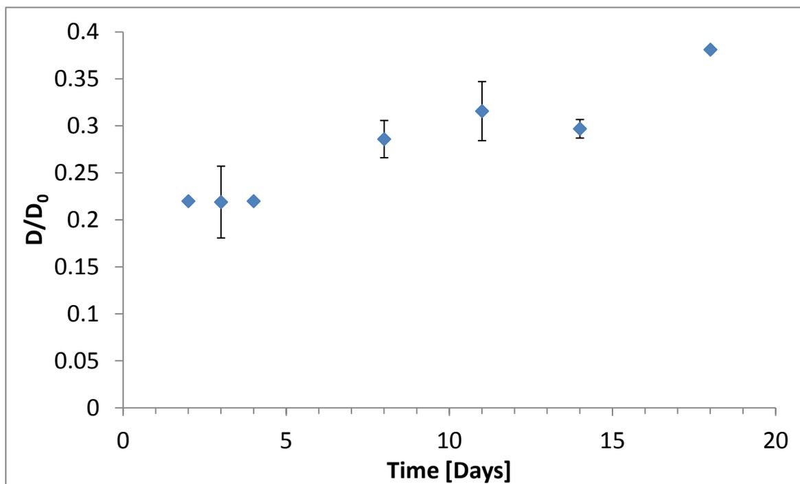
**Figure 9.11: Normalised diffusion coefficient at 300 ms at a temperature of 65°C.**
