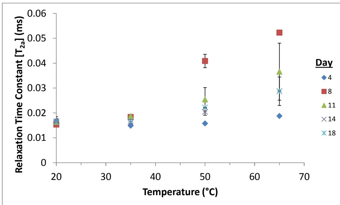
Figure 9.4: Change in the relaxation time constant for the water associated with protein within Mozzarella during heating and storage. (Error bars =  $\pm 1$  standard deviation).
