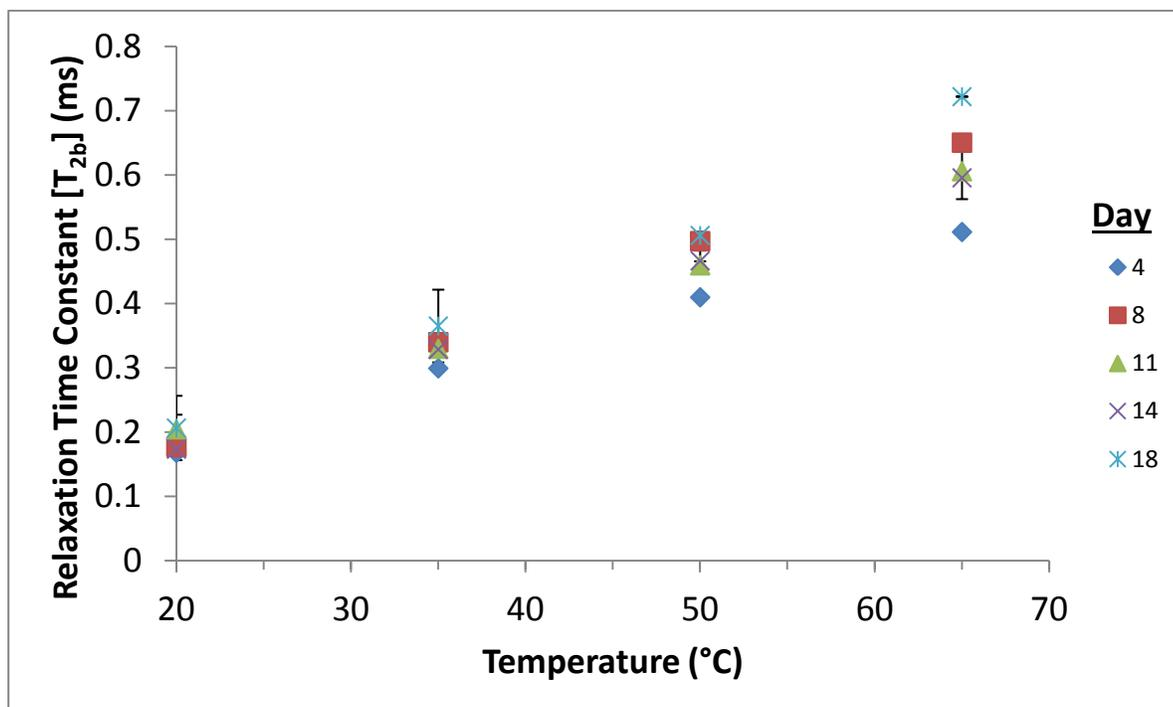
Figure 9.3: Change in the relaxation time constant for the free water in Mozzarella with temperature and storage. (Error bars =  $\pm 1$  standard deviation).
