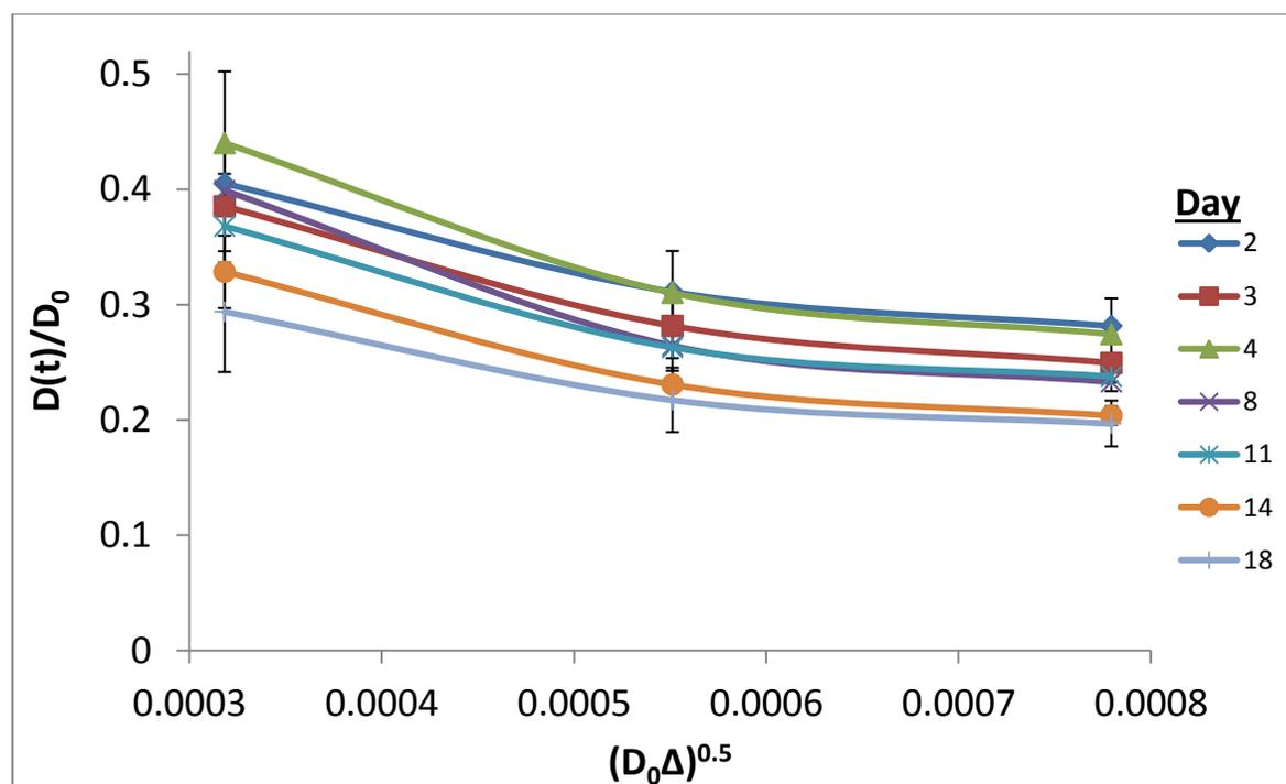
Figure 9.5: Diffusion coefficients of water at 20°C over the storage trial measured using a stimulated echo PGSE sequence in the transverse direction as a function of the observation time. The diffusion coefficients are normalised using the diffusion of free water at 20°C estimated at  $D_0 = 2.03 \times 10^{-9} \text{ m}^2 \text{ s}^{-1}$ .
