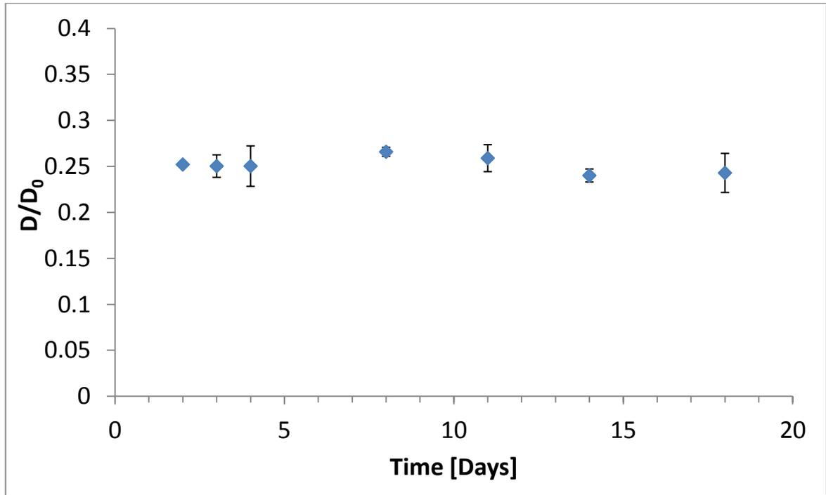
Figure 9.9: Normalised diffusion coefficient at 300 ms at a temperature of 35°C.
