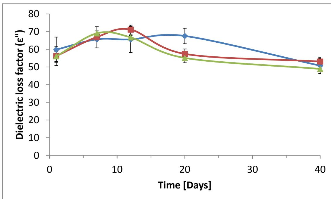
Figure 10.20: Change in the dielectric loss factor over the storage trial at 244 MHz [◆ Low (129), ■ Control (148) and ▲ High (171)].
