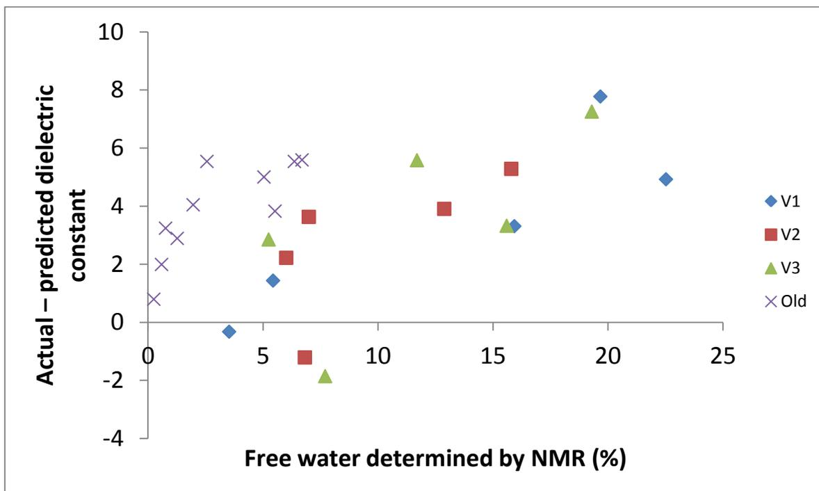
Figure 10.22: Difference in the actual and predicted dielectric constant versus free water determined by NMR [◆Low (129), ■ Control (148) and ▲High (171) and X data from Chapter 6].
