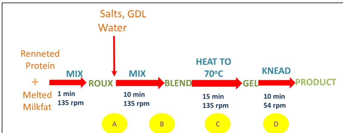
Figure 4.1: Model system manufacturing process
