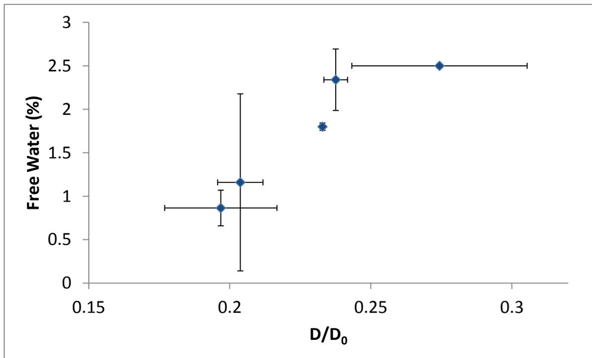
Figure 9.6: Relationship at 20°C between the quantity of free water in the sample and the normalised diffusion coefficient at 300 ms.
