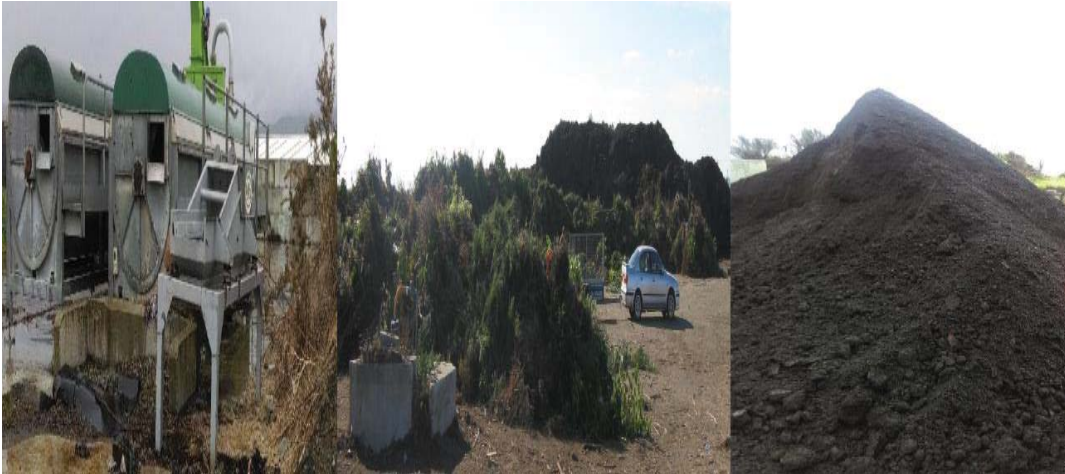
Figure 1 Commercial composting at the Awapuni composting site (Hot Rot in-vessel composting system (left), garden waste drop-off (middle) and finished compost (right). Source: (Hannon, Hay, City Enterprises, Allen, & Simmons, 2014).
