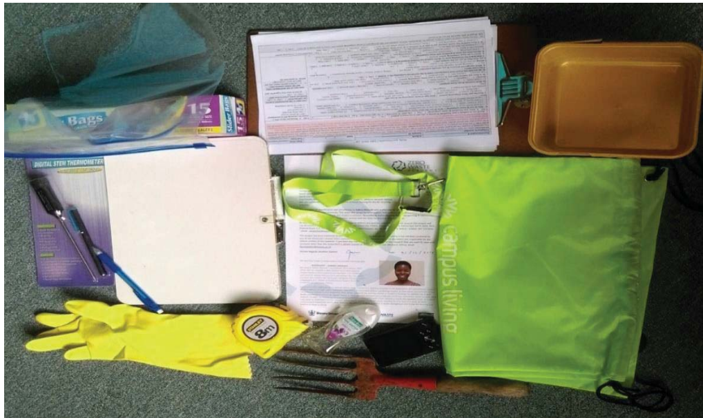
Figure 14 Apparatus for the collection of compost samples during home visits in the present study. They comprised: temperature probe, two-litre fixed container, zip-lock bags, digging fork, white marker board, camera, gloves, tape measure, identification card)
