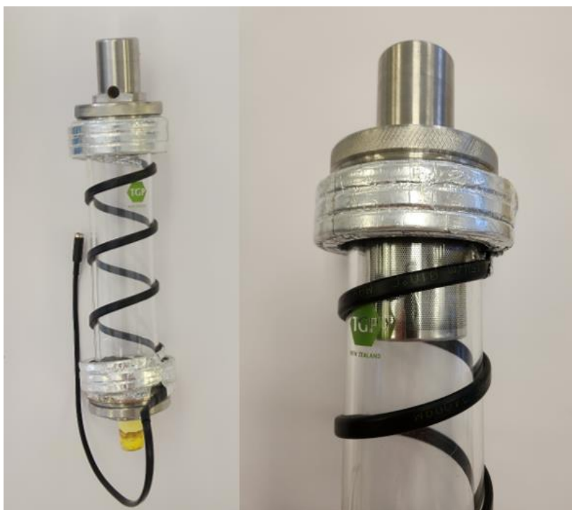
Figure 13A and 13B: Shows the reactor column used to house the botanical basket, the column is wrapped in heat trace. The stainless-steel caps are also visible at either end of the column. The botanical basket is also visible within the column on the right.
