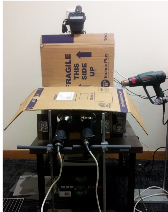
Figure 7.3 Experimental setup and oven modifications showing lighting arrangement
