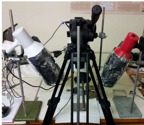
Figure 3.5 – The experimental setup for lighting, heating and image capture during cheese browning trials
