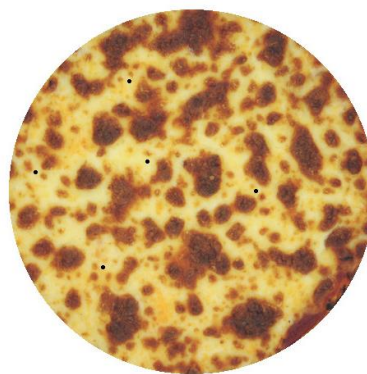
Figure 5.11 – Visual representation of a minimum blister size of 20 pixels (black dots represent 20 pixels, equivalent to 2.2mm diameter wide blister)
