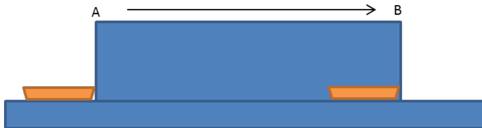
Figure 4.15 – Illustration of points used to measure bake time from the entry to the oven (A) to the exit of the oven (B)
