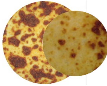
Figure 7.32 – Relative area assessed for commercial oven experiments (left image) compared to benchtop oven experiments (right image)
