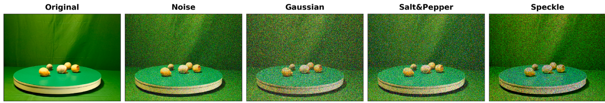
Fig. 15. Examples of the implemented noise types. Applied to RGB3; columns show Original, Noise, Gaussian, Salt & Pepper, and Speckle.
