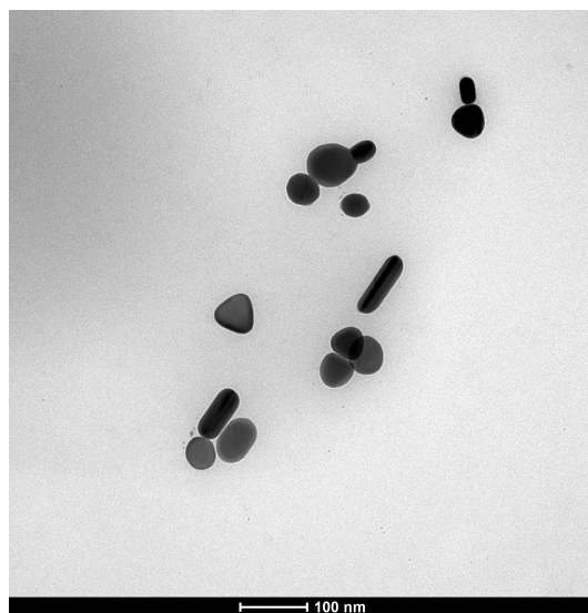
Figure 5.10: TEM image showing the various particle geometries found in a nanorod preparation with a \gamma value of 4
