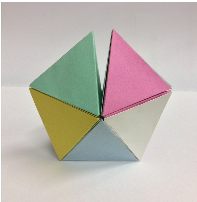
Figure 1.3: Origami representation of the penta-twinned seed particles made up from 5 tetrahedra. The five twin-planes can also be seen where the faces of each tetrahedra meet
