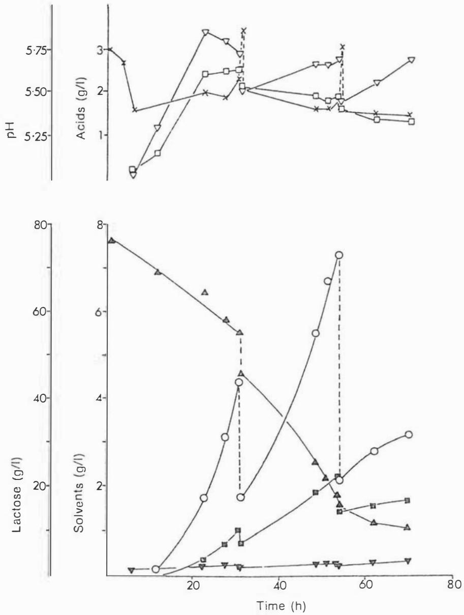
Figure 9.2. Fermentation profile for the adsorption resin (XAD-16) - solvents recovery from a batch fermentation using sulphuric acid casein whey permeate medium. Symbols as for Fig. 9.1.
