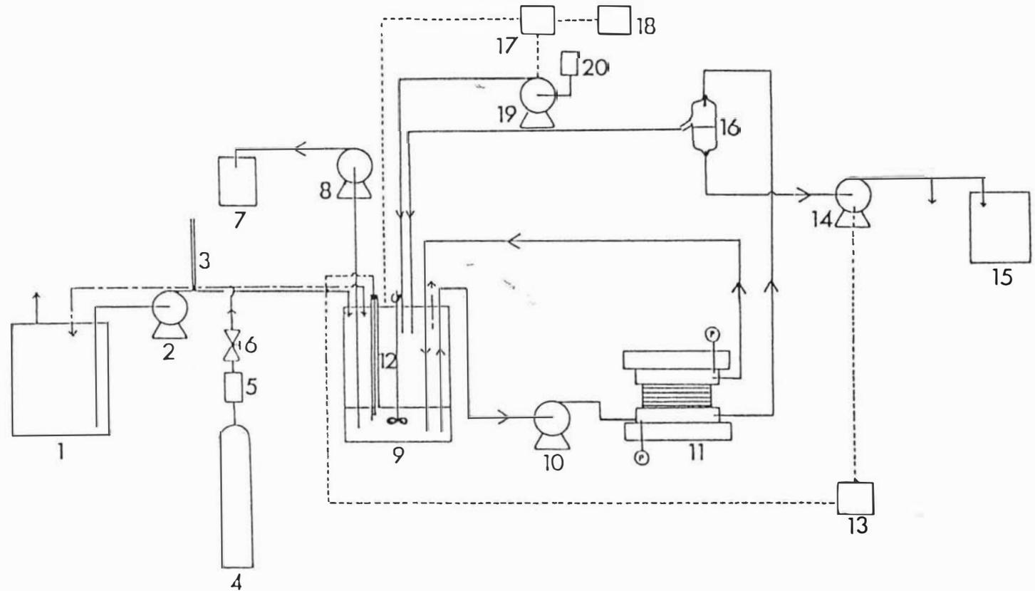
Figure 3.5. A schematic diagram of the fermenter and ancillary equipment used for continuous fermentation using external cell recycle with a Millipore<sup>®</sup> Plate and Frame cross-flow microfiltration (CFM) unit.
