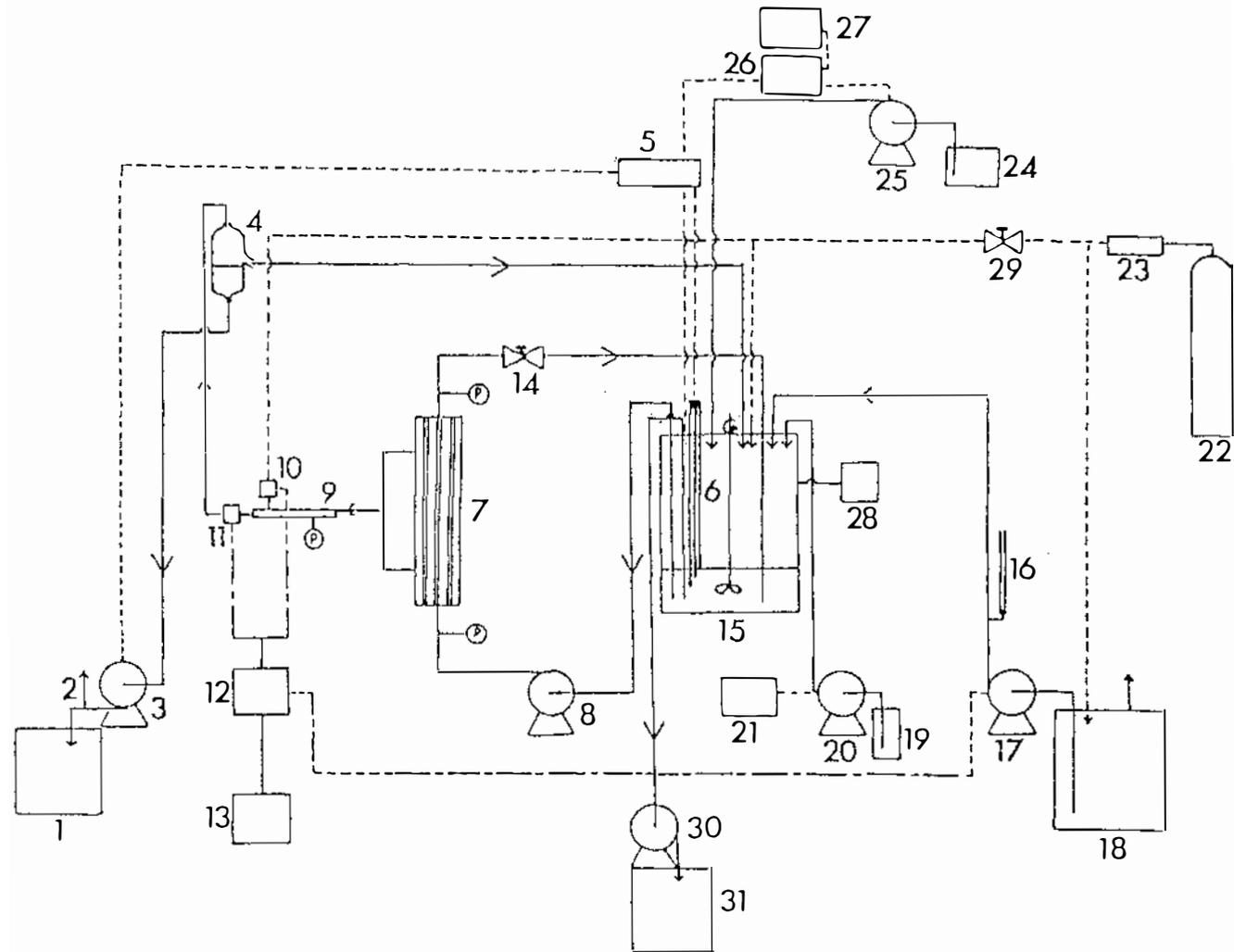
Figure 3.7. A schematic diagram of the fermenter and ancillary equipment used for continuous fermentation using external cell recycle with a Cerallo<sup>®</sup> Tubular cross-flow microfiltration unit.
