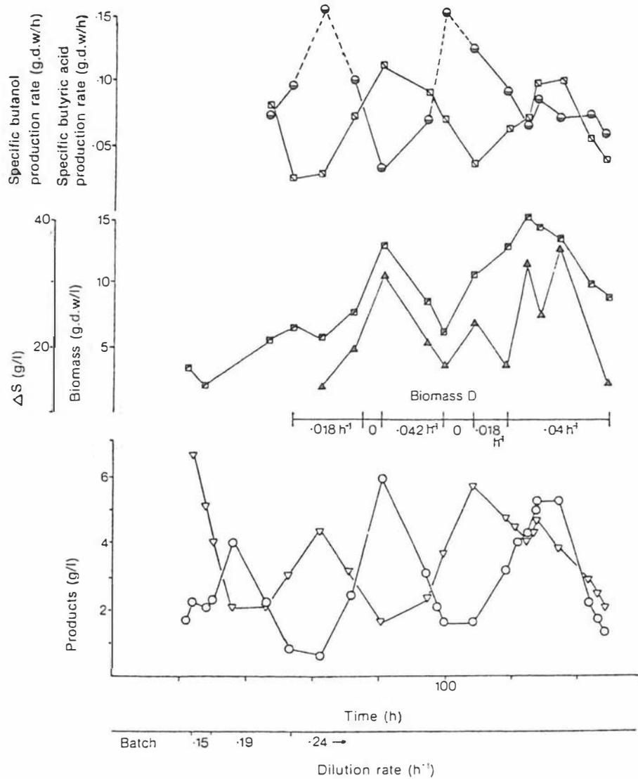
Figure 7.7. Continuous fermentation profile of Run VII (34°C, Tubular CFM apparatus). Symbols as for Fig. 7.5.
