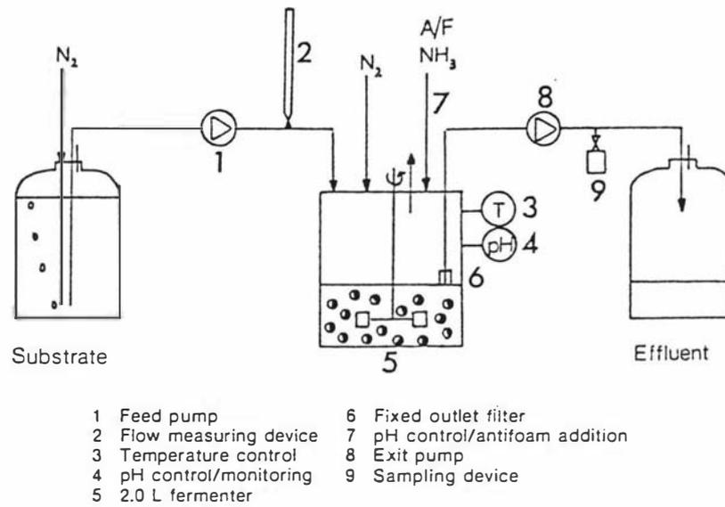
Figure 3.2. A schematic diagram of the continuous stirred tank reactor and ancillary equipment used with immobilized cells.
