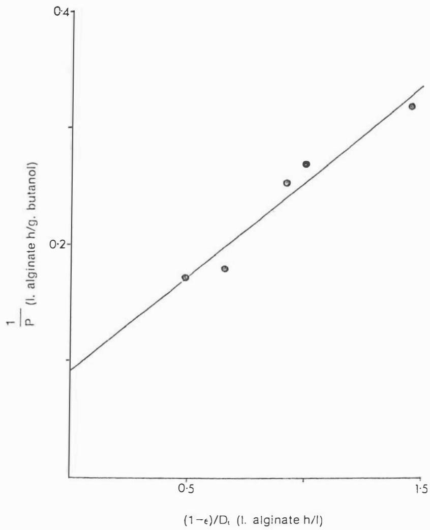
Figure 6.7. Double reciprocal plot of  $P$  vs  $D_i/(1-\epsilon)$  using data derived from Table 6.4 for semi-synthetic medium containing glucose.
