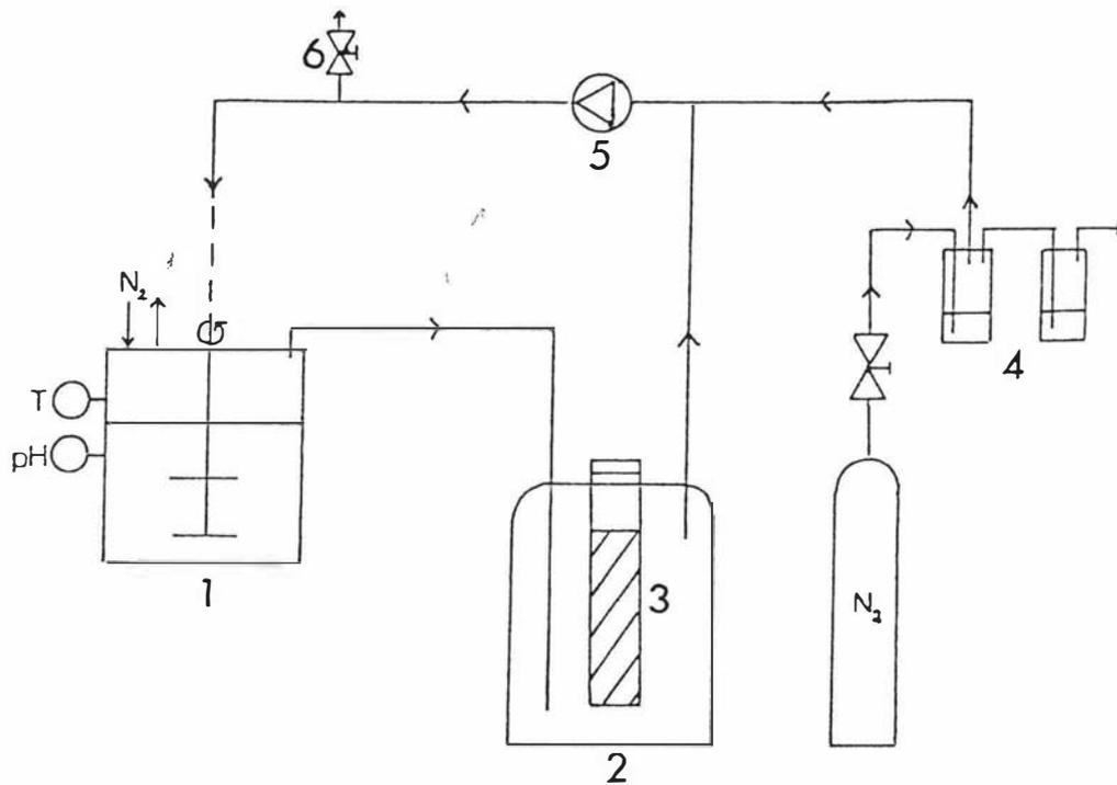
Figure 3.9. A schematic diagram of the integrated batch fermenter - gas stripping/condensation apparatus. 1 fermenter; 2 condenser; 3 cold finger; 4 gas inlet/outlet; 5 gas recycle pump; 6 gas exit.
