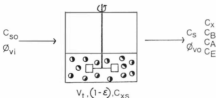
Figure 2.3. A schematic diagram of the immobilized cell system showing those measurable parameters necessary for the kinetic model parameter estimation.
