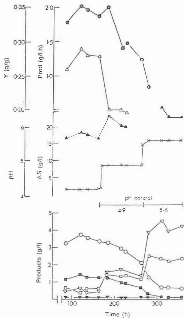
Figure 6.5. The effect of pH control on a continuous fermentation using immobilized *C. acetobutylicum* at 30°C using cheese whey permeate medium supplemented with 20 g/l lactose. ( $(1-\epsilon) = 0.25$ ,  $D_c = 0.40 \text{ h}^{-1}$  or  $0.44 \text{ h}^{-1}$ ). Run XIV. Symbols as for Fig. 6.1
