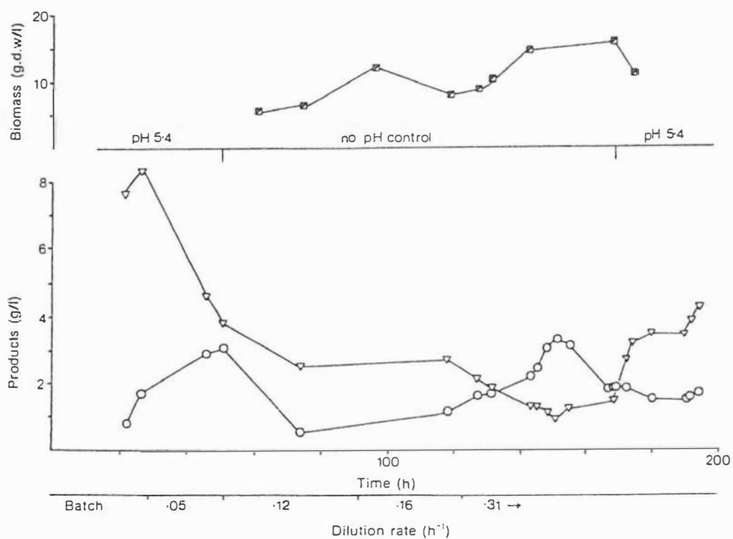
Figure 7.1. Continuous fermentation profile of Run 1 (complete biomass recycle, 30°C, Plate and Frame CFM apparatus, Durapore cassette): (O) butanol; ( $\nabla$ ) butyric acid; ( $\blacksquare$ ) biomass concentration.
