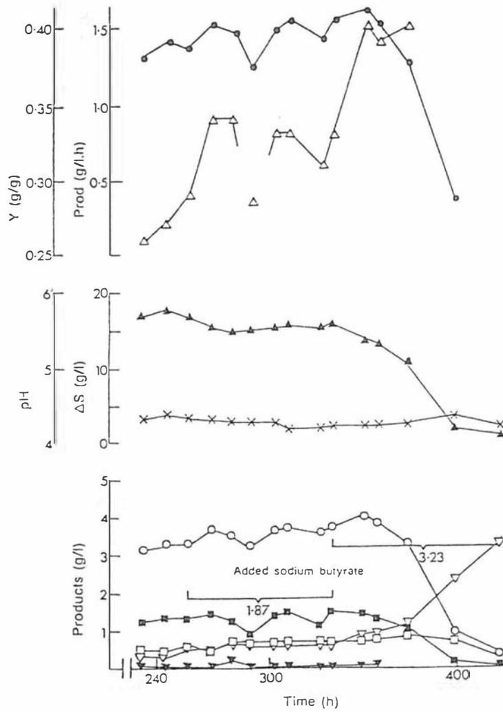
Figure 6.6. The effect of added butyrate (pH 4.6) on a continuous fermentation using immobilized *C. acetobutylicum* at 30 °C ( $(1 - \epsilon) = 0.25$ ,  $D_i = 0.29 \text{ h}^{-1}$ ). Run XV. Symbols as for Fig. 6.1.
