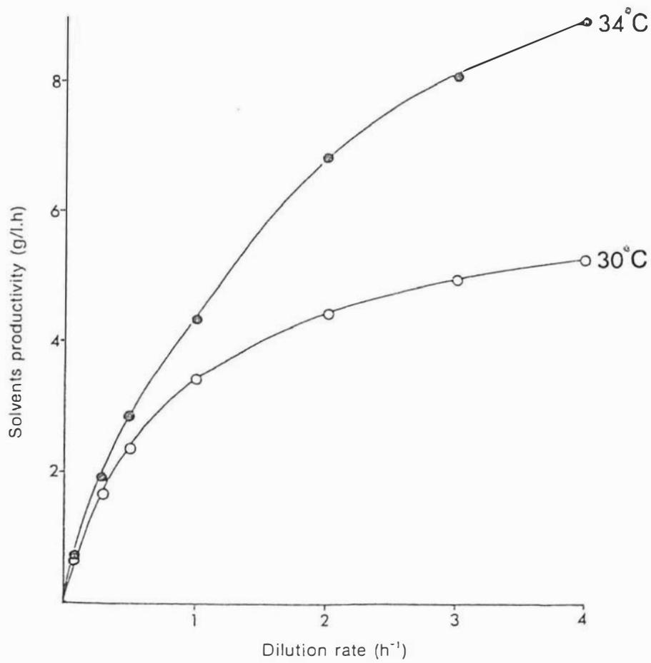
Figure 6.10. The solvents productivity (g/l.h) calculated as a function of the dilution rate for a reactor loading  $(1-\epsilon)$  of 0.45, using kinetic parameters derived in Section 6.2.4 for cheese whey permeate.
