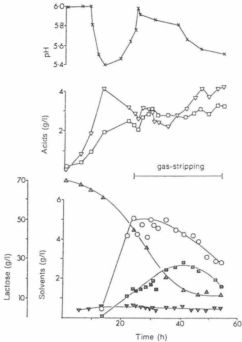
Figure 9.1. Fermentation profile for the gas-stripping/condensation solvents recovery from a batch fermentation using sulphuric acid casein whey permeate medium: (○) butanol; (■) acetone; (▼) ethanol; (▽) butyric acid; (□) acetic acid; (x) pH; (▲) lactose.
