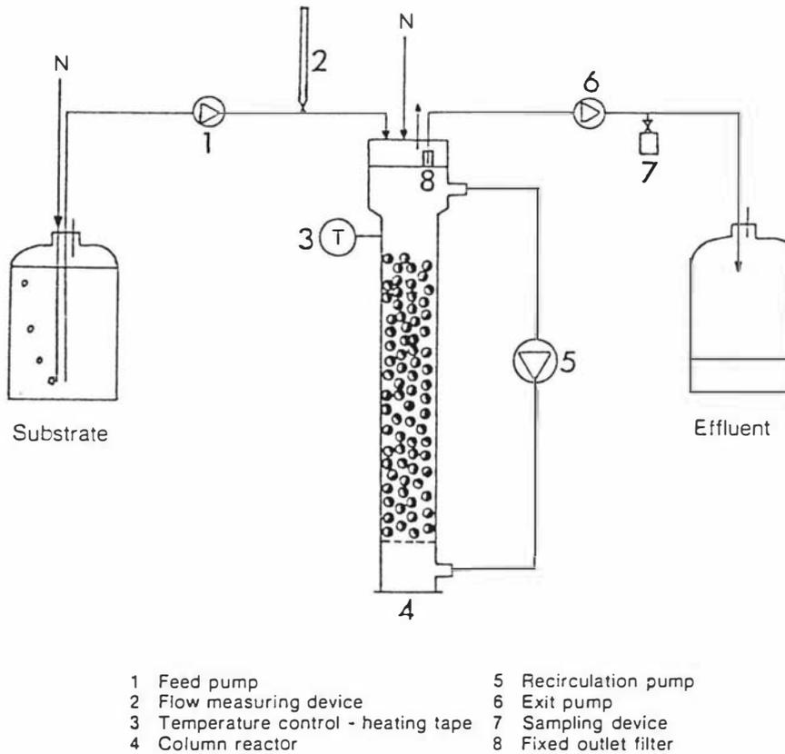
Figure 3.3. A schematic diagram of the fluidized column reactor and ancillary equipment used with immobilized cells.
