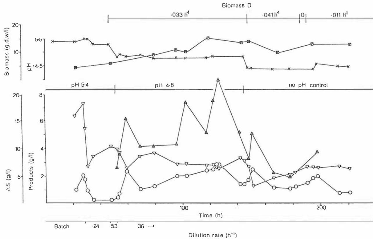
Figure 7.2. Continuous fermentation profile of Run II (biomass removal, 30°C, Plate and Frame CFM apparatus, Durapore cassette): (O) butanol; ( $\nabla$ ) butyric acid; (■) biomass concentration; (▲) substrate utilization; (x) pH.
