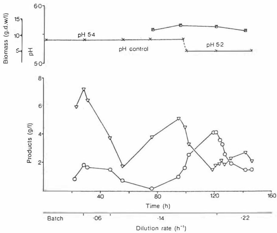
Figure 7.5. Continuous fermentation profile of Run V (30°C, Hollow Fibre CFM apparatus). Symbols as for Fig. 7.1.
