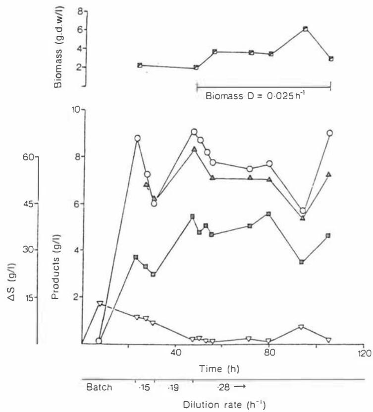
Figure 7.4. Continuous fermentation profile of Run IV (semi-synthetic medium containing glucose, 34°C. Plate and Frame CFM apparatus, Ultrasart cassette). Symbols as for Fig. 7.2; (■) acetone.
