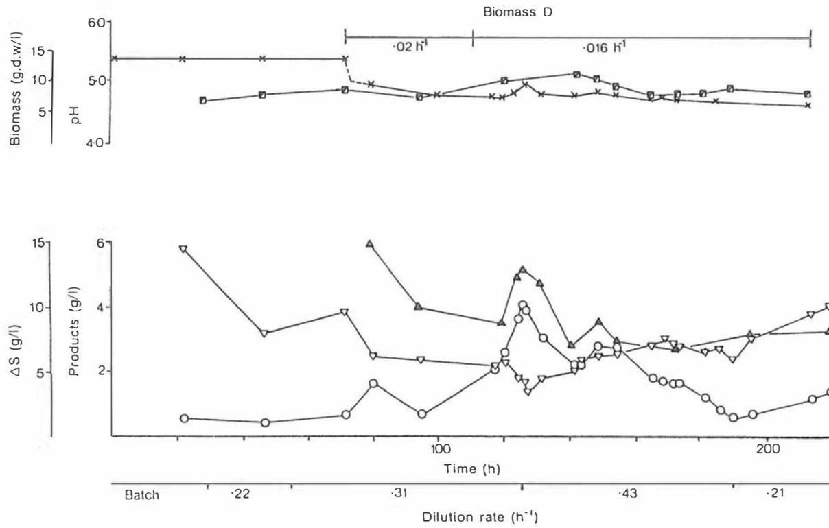
Figure 7.3. Continuous fermentation profile of Run III (30°C, Plate and Frame CFM apparatus, Ultrasart cassette). Symbols as for Fig. 7.2.
