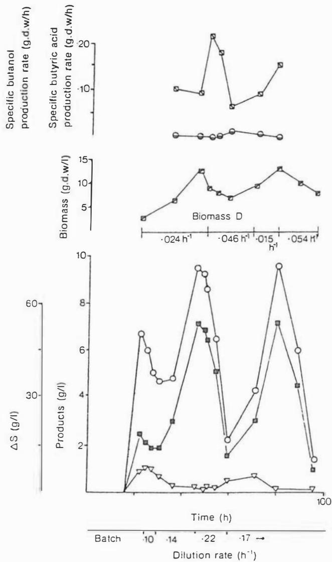
Figure 7.6. Continuous fermentation profile of Run VI (semi-synthetic medium containing glucose, 34 °C, Tubular CFM apparatus): (○) butanol; (■) acetone; (▽) butyric acid; (■) biomass concentration; (▲) substrate utilization; (⊞) specific butanol production rate; (⊕) specific butyric acid production rate.
