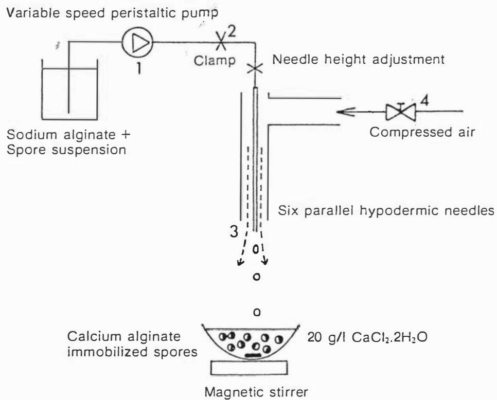
Figure 3.1. A schematic diagram of the immobilization equipment.
