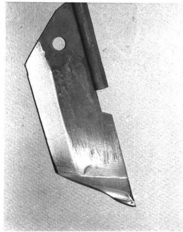
Figure 54: Trash collecting hook of hardened material (EutecBor).
