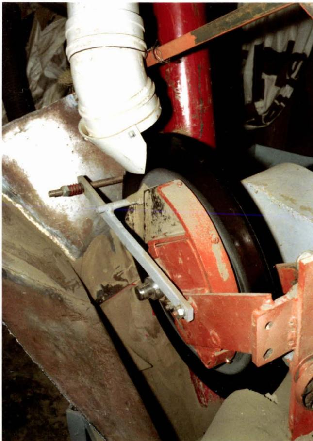
Figure 6: The calibrated spring tensioner used to simulate the lateral soil pressure measured against the coulter blade in the Pilot Test.
