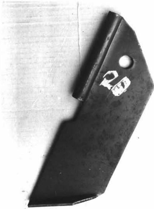
Figure 14b: Run A: Carbonitrided mild steel blade.
