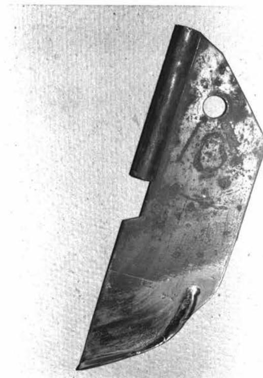
Figure 53: Field wear of chromium plated mild steel in Run B.
