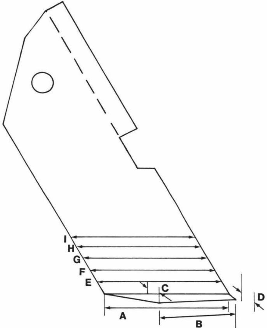
Figure 12: The measurement jig that was used for standardising coulters linear measurements.
