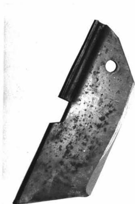
Figure 23: Soil 1: In the absence of soil, the blade sustained a markedly reduced wear rate compared with the soil situation.
