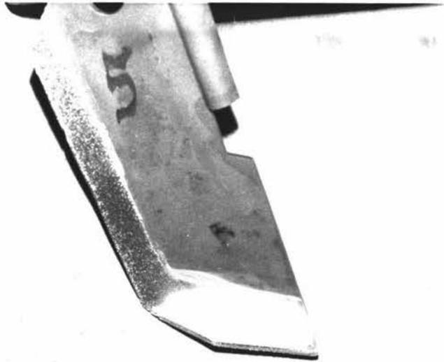
applications developed prematurely a trash-collecting hook of hardened material. This was due to the thinner weld bead eroding essentially parallel to the leading edges of blade wings. The initial breakthrough-point caused trash to collect because of differential wear of the bead and the softer base material adjacent to it.
