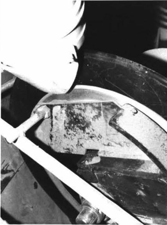
Figure 19: Although 10 hours continuous operation had elapsed, the metal surface of the blade had barely been disturbed where soil had been absent.
