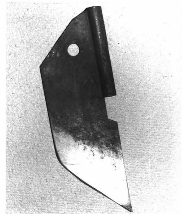
Figure 43: Field wear of carbonitrided mild steel blades in Run A.
