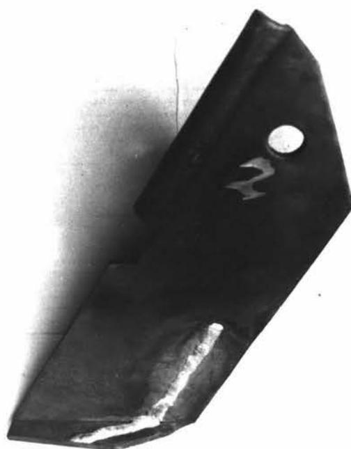
Figure 34: Bottom weld bead pattern design for coulter blades used in Run A of Experiment 3.
