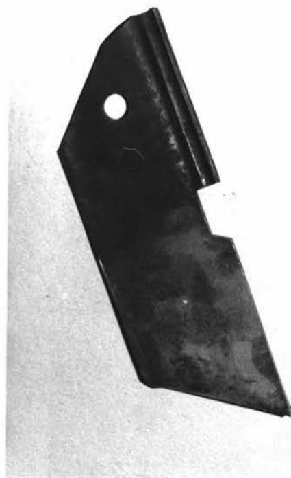
Figure 24: Soil 2: Where soil was present, the two regions of different wear were evident on the disc.
