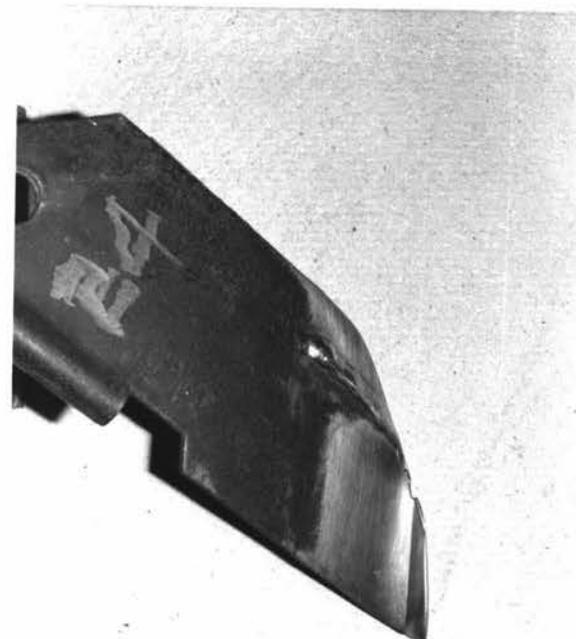
Figure 45: Field wear of Toolcraft (-bottom pattern) welded over mild steel in Run A.
