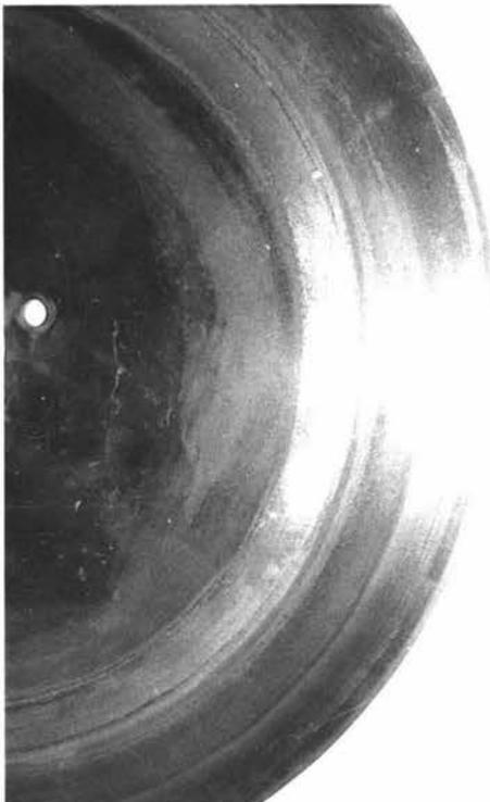
Figure 22: Soil 1: On the soil side, both wear mechanisms were evident throughout the length of the inner blade leading edge. The lower grey area corresponded to the soil contact zone, while the upper portion was not in soil contact.
