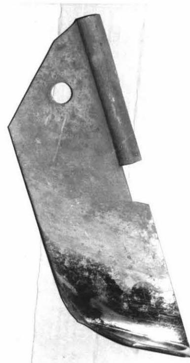
Figure 50: Field wear of Eutalloy Tungtec welded over mild steel in Run B.
