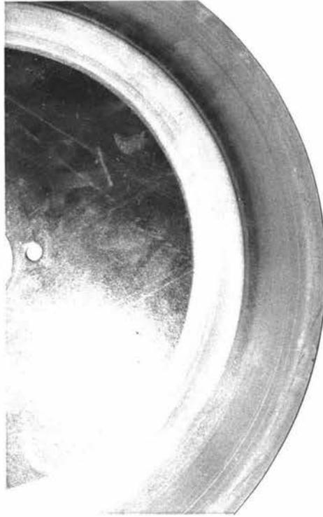
Figure 21: In the absence of soil, wear appeared to be adhesive within the contact width, as shown by the blotchy and shiny surface.
