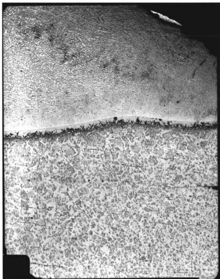
The microstructure of chromium plated mild steel can be seen in Figure 41h. Since only stress relief of the plates was carried out, there was not sufficient heat to transform the base plate microstructure. Electroplating thickness was about 0.1mm. and the hardness measured (Figure 40h) was only at the lower range of that claimed for chromium (HV=850-1040).
