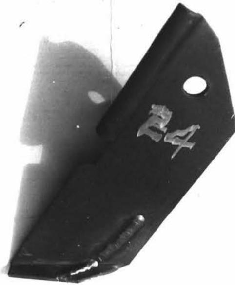
Figure 14d: Run A: Toolcraft arc welded over mild steel -bottom pattern.
