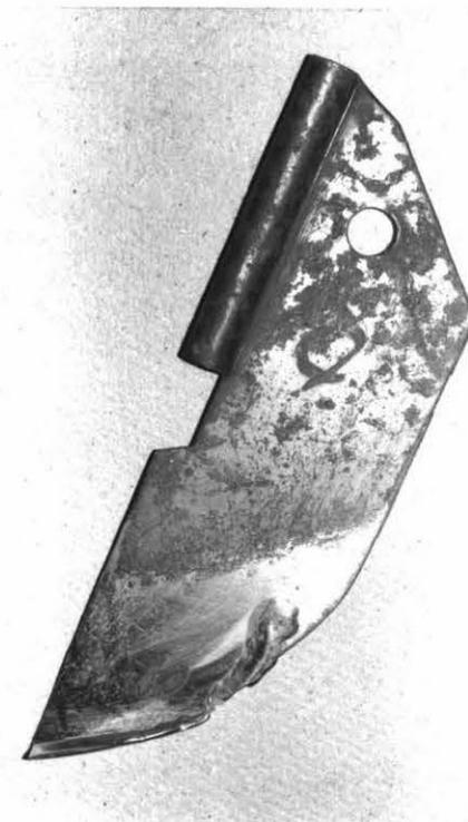
Figure 52: Field wear of Ultimum welded over mild steel in Run B.
