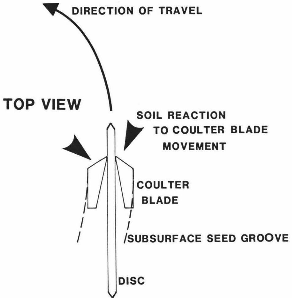
reaction on the inside of the disc was likely to have been lower than that on the outside. During field operation, increased soil reaction while turning corners was evident as a larger, more shattered seed groove on the outside of the disc.
