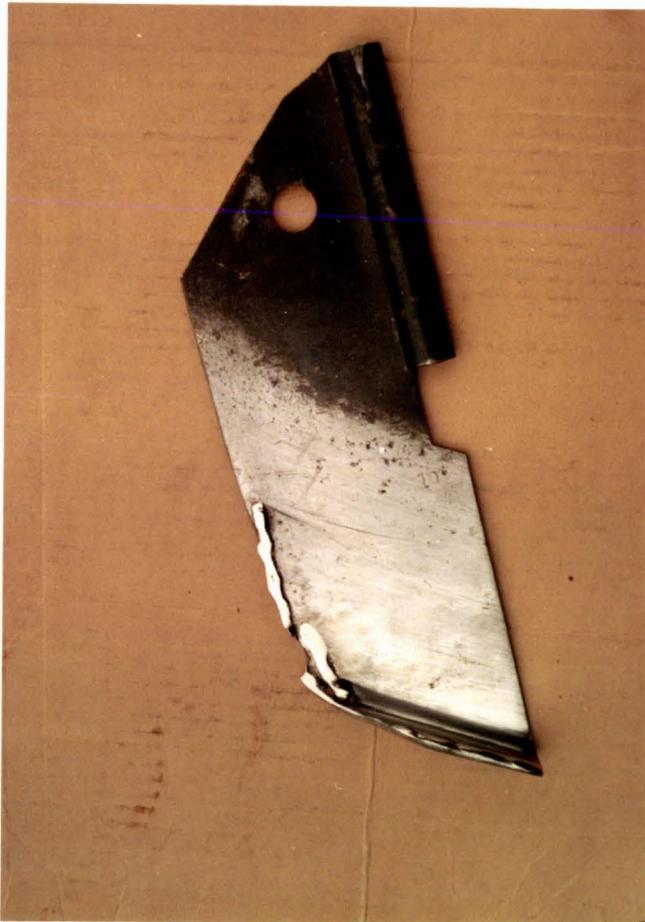
Figure 32: The reverse side of the blade in Figure 31 showing the chip out of the leading edge.
