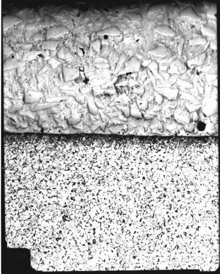
quantified that property of the matrix. The third measurement (HV=1390) is likely to have been the hardness of an individual tungsten carbide particle. Claimed general hardness for this material was HV=650 to HV=850. No explanation is apparent for the measured matrix hardness having been greater than the claimed general hardness.
