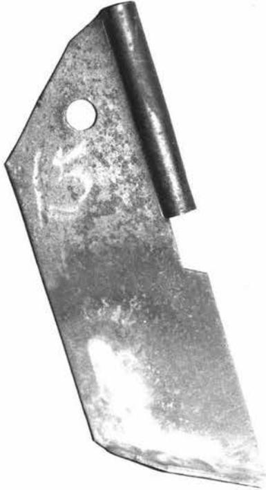
Figure 15b: Run B: Cobalarc arc welded over mild steel.
