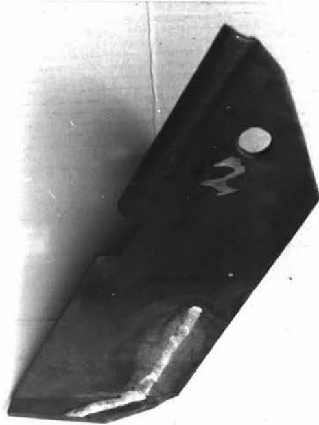
Figure 14f: Run A: EutecBor gas welded over mild steel -bottom pattern.
