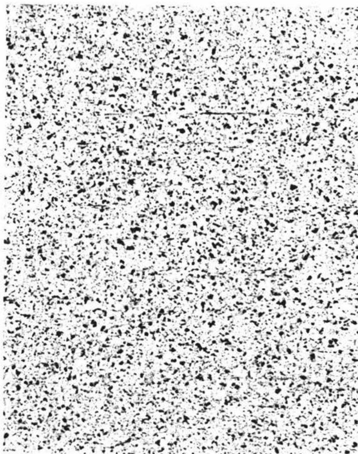
ferrite predominate over the pearlitic regions (darker) due to the carbon content of this alloy (0.19%) not being sufficient to have allowed all of the austenite to decompose to pearlite. Pearlite has a fine grained structure in this situation, which suggests that the steel had been normalised during manufacture (air cooled from the austenitic range). Surface hardness was HV=177 (Figure 40b), which was considerably softer than the disc component upon which the coulter blades were impinging.
