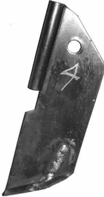
Figure 15d: Run B: Chromium plated mild steel.
