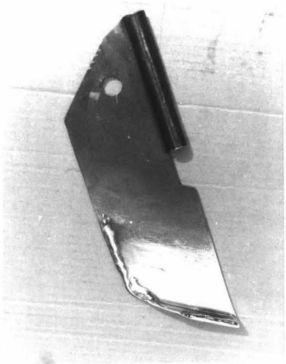
contrast to the standard blades which eventually were worn in a curve simulating disc rotation against the inner leading edge. This interaction between the disc and the blade is illustrated in Figures 29 and 32. The disc tended to transport soil over the blade leading edge in a pattern clearly shown in the photographs. The result was that the blade leading edge was worn to the shape of the disc radius, inevitably accelerating wear of the coultter wing in the process.
