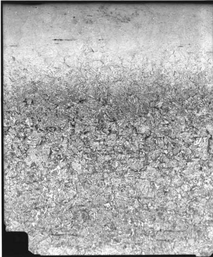
above that for mild steel. Surface hardness was also higher than claimed (HV=836) and the hardened region extended further (1.00mm.) than the claimed case depth (0.51mm.).
