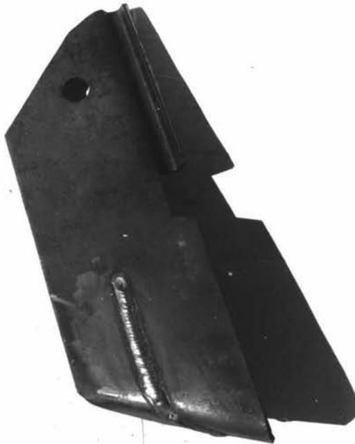
Figure 14e: Run A: EutecBor gas welded over mild steel -top pattern.
