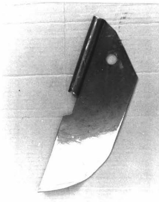
Figure 28d: Field wear of a treated blade after 20 km. (4.8 ha.) drilling.
