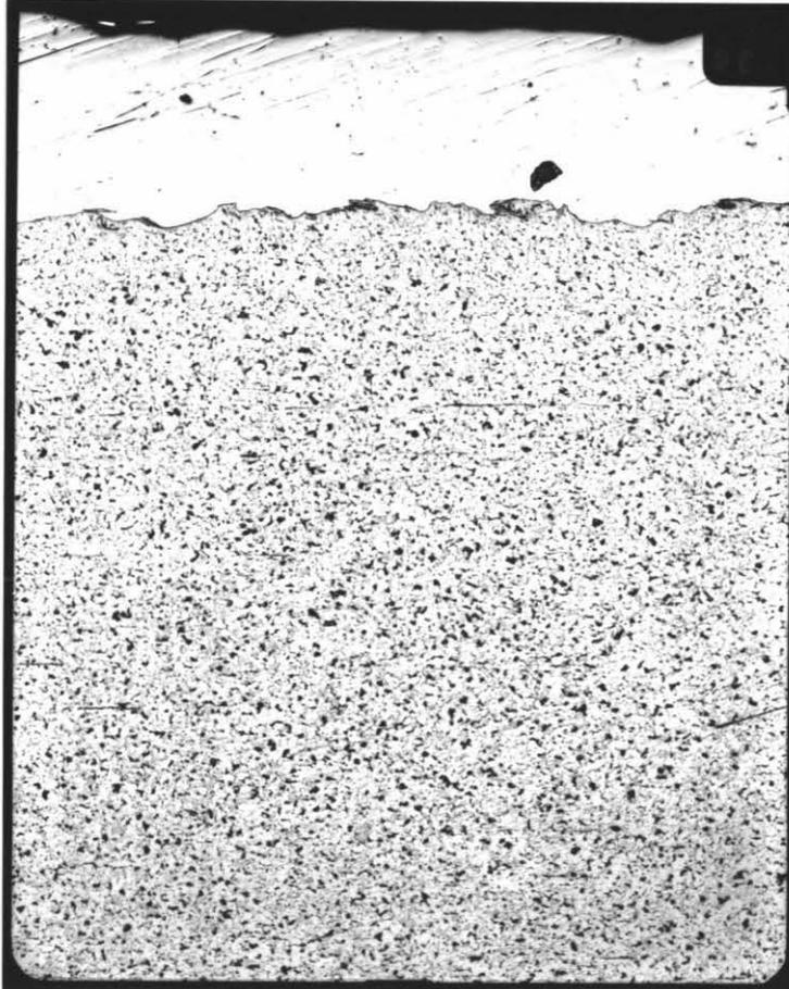
Figure 41i: Microstructure of arc welded Toolcraft from the weld surface (top) to mid cross-section of the base plate. (Nitral, 88x)
