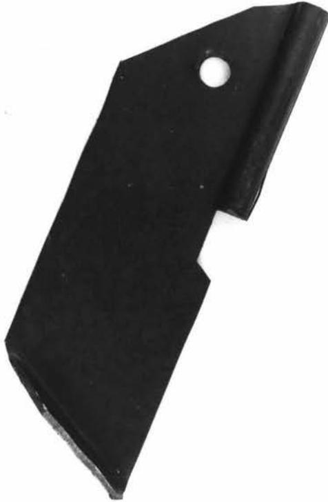
Figure 10: Typical hardfacing deposit over a mild steel coultter blade.
