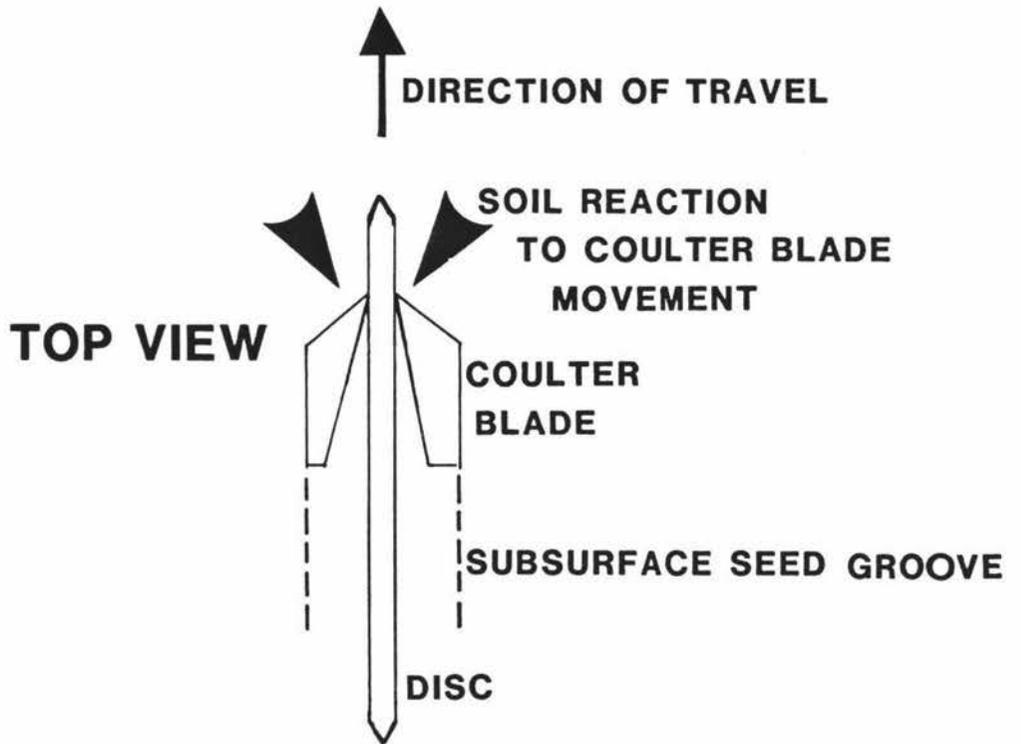
Figure 39b: Diagram illustrating the probable soil reaction forces to coulter assembly travel during cornering.
