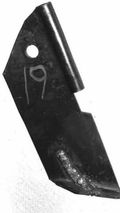
Figure 15c: Run B: Ultimum arc welded over mild steel.
