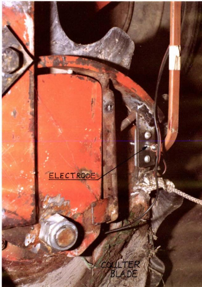
Figure 4: The single coulter assembly on the three row testing rig. The indicator light can be seen at the middle of the right hand side. The pulley reduction is not shown.
