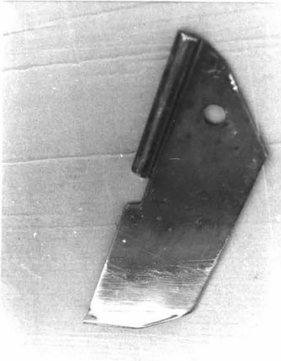
Figure 28b: Field wear of a standard blade after 90 km. (21.6 ha.) drilling.
