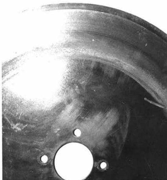
Figure 26: Soil 2: Where soil was present, the two regions of different wear were evident along the inner leading edge of the blade.
