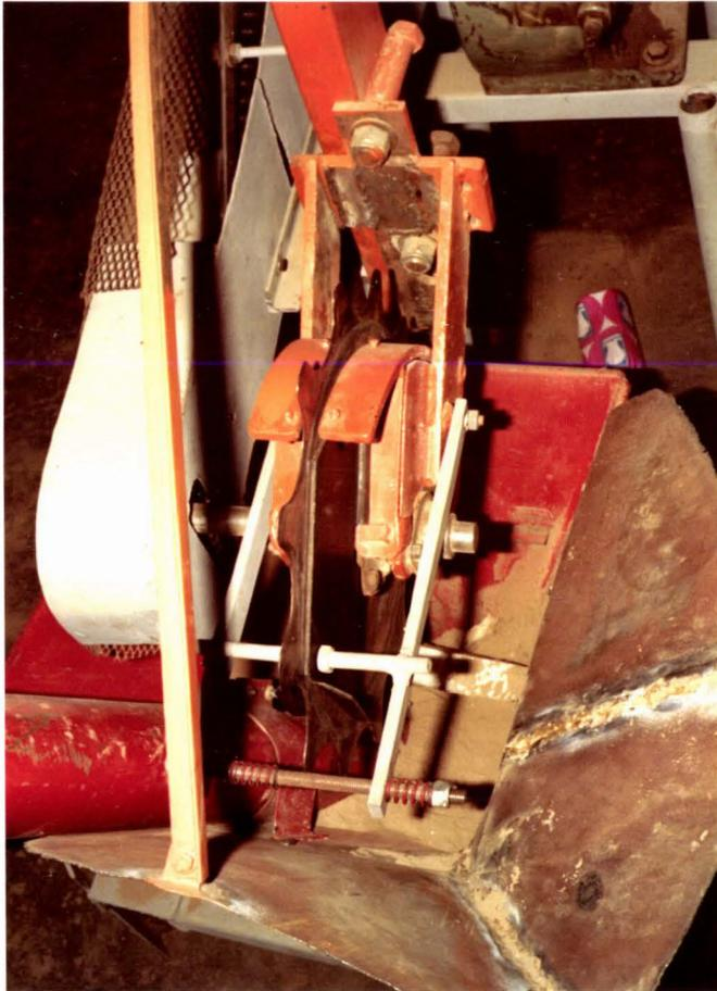
variable in the range 100 to 800 rpm. This gave a theoretical ground speed range of 2.8 to 22.6 km/hr. Tests were carried out at an equivalent ground speed of 5 km/hr.
