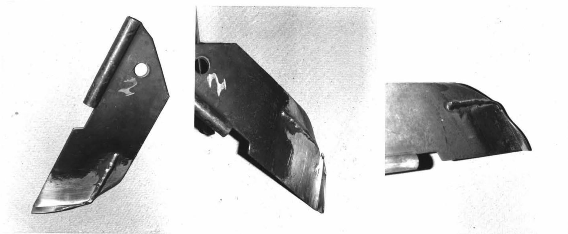
Figure 47: Field wear of EutecBor (-bottom pattern) welded over mild steel in Run A.
