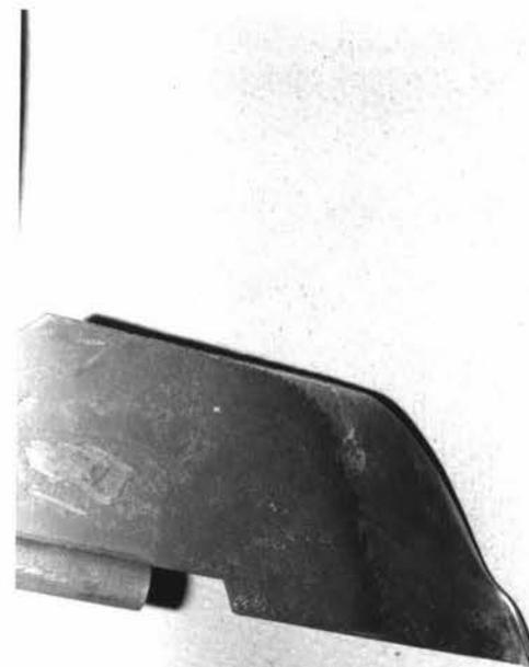
Figure 49: Field wear of carbonitrided mild steel blades in Run B.
