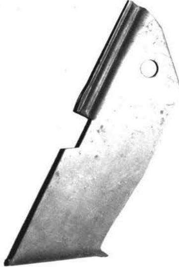
Figure 27: Soil 2: In the absence of soil, wear was markedly reduced compared to both the "soil" situation for Soil 2 and the "no soil" situation for Soil 1.
