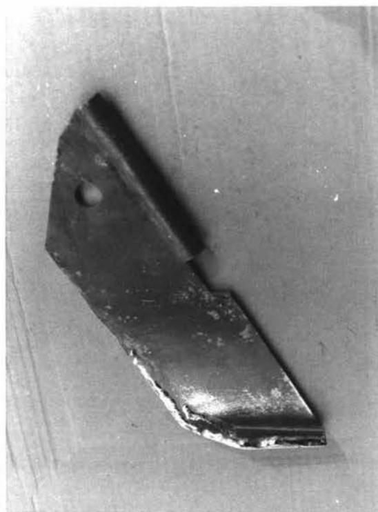
Figure 28e: Field wear of a treated blade after 90 km. (21.6 ha.) drilling.
