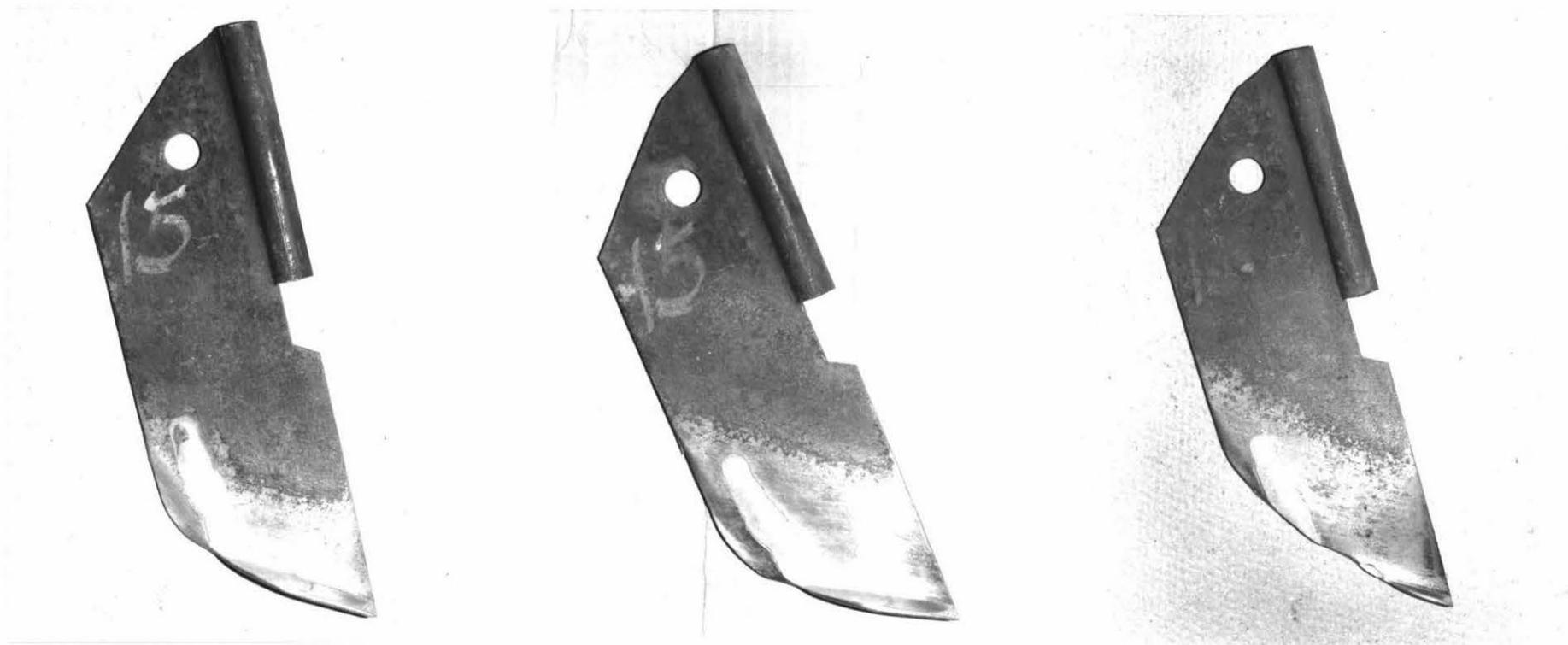
Figure 51: Field wear of Cobalarc welded over mild steel in Run B.
