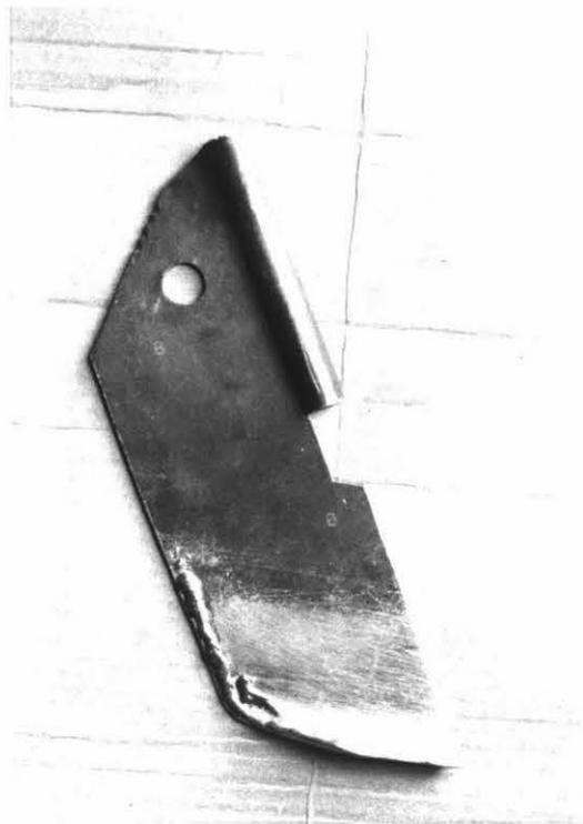
Figure 28f: Field wear of a treated blade after 190 km. (45.6 ha.) drilling.
