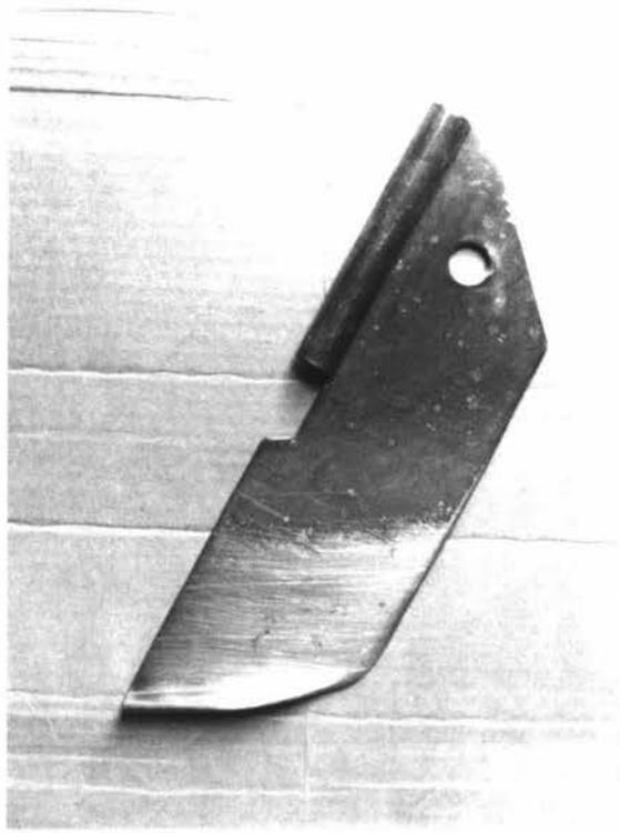
Figure 28c: Field wear of a standard blade after 190 km. (45.6 ha.) drilling.
