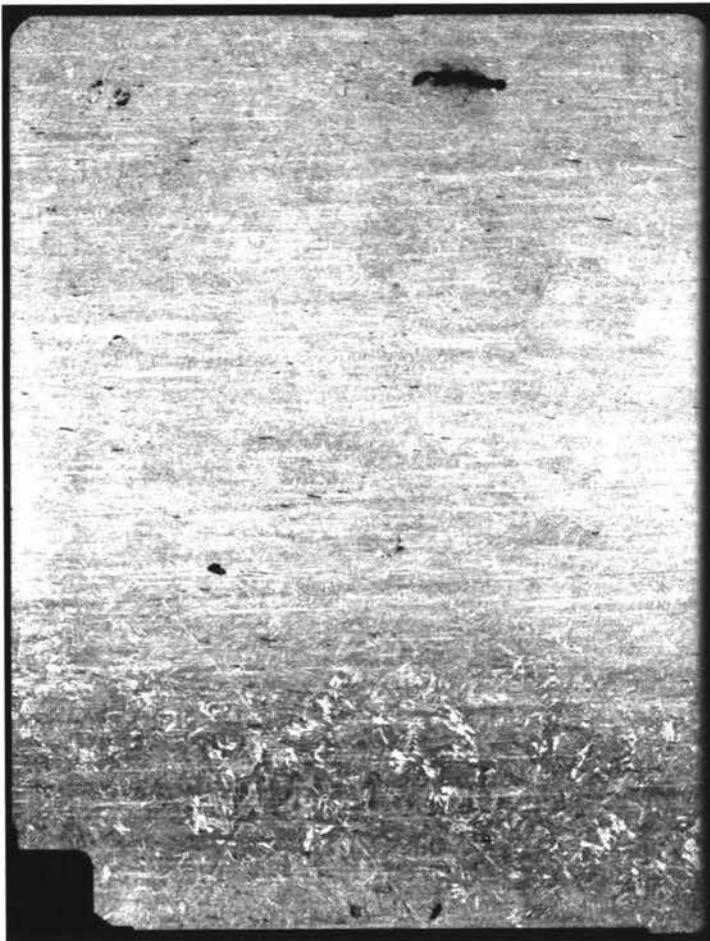
Figure 41b: Microstructure of mild steel. (Nitral, 88x)
