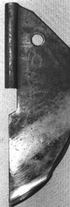
Figure 44: Field wear of Toolcraft (-top pattern) welded over mild steel in Run A.
