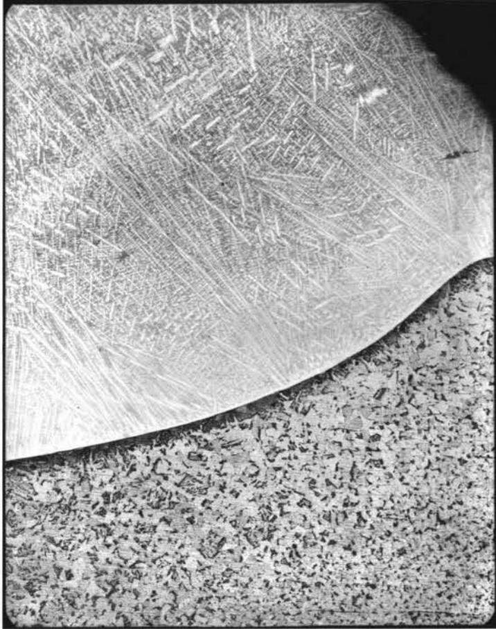
Figure 41f: Microstructure of gas welded Tungtec from the weld surface (top) to mid cross-section of the base plate. (Nitral, 88x)
