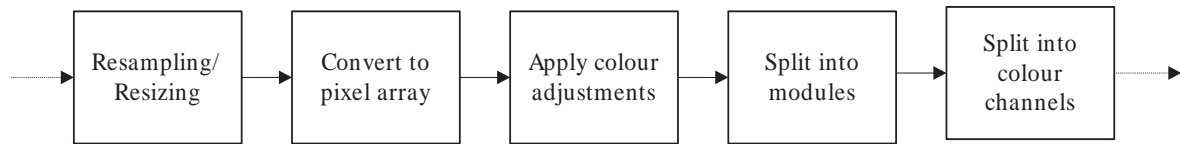
Figure 33 - Software processing steps
