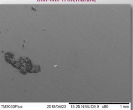
Figure 9: SE topographical distribution of 25 μm thin-film Ti membrane after 160 million cycles
