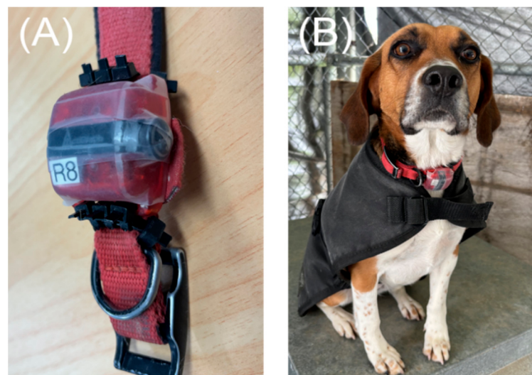
Figure 1. Accelerometer placement and coat fitting showing (A) a close-up view of the accelerometer wrapped in waterproof tape and fixed to a collar, and (B) a dog fitted with the coat and collar-mounted accelerometer.
