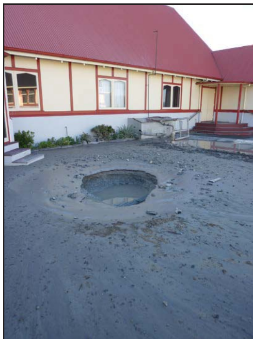
Figure 2 St. Faith's church (Rotorua) hydrothermal explosion deposits in 2011, caused by the leakage of a bore, seen below the window on the right-hand side. Photo by A. Somerville.
