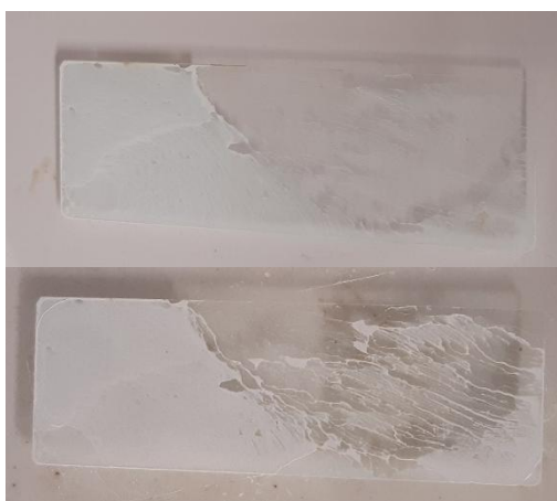
Figure 4.1 Initial TiO 2 coating test with one layer (top) and two layers (bottom) deposited. Adding extra layers dissolved the preceding layers.
