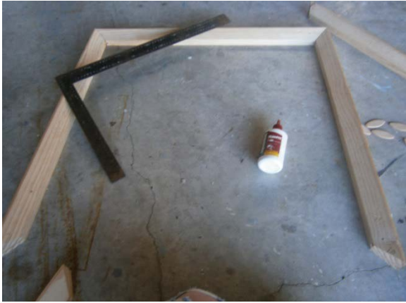
Figure 9 Making the stretcher frame
