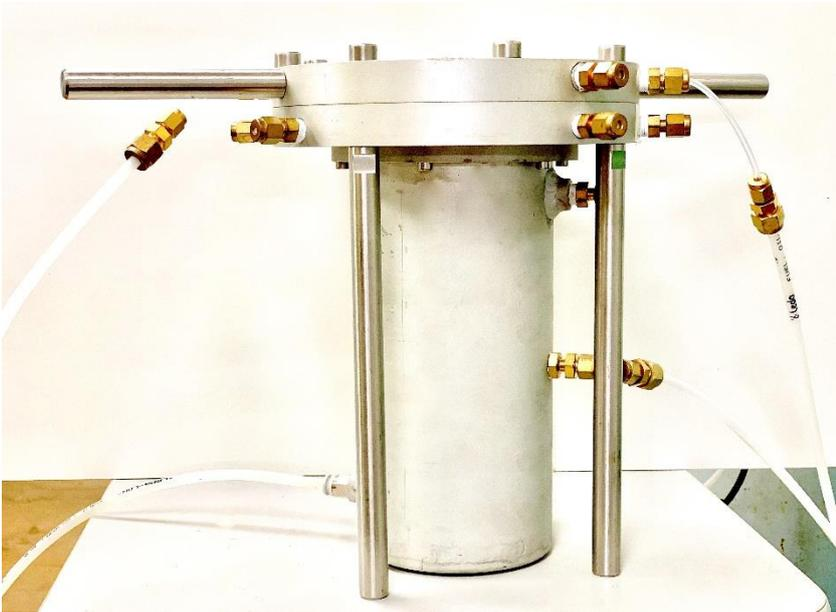
**Figure 4.2** Permeability cell (ID = 0.1 m) used in film permeability measurement.
