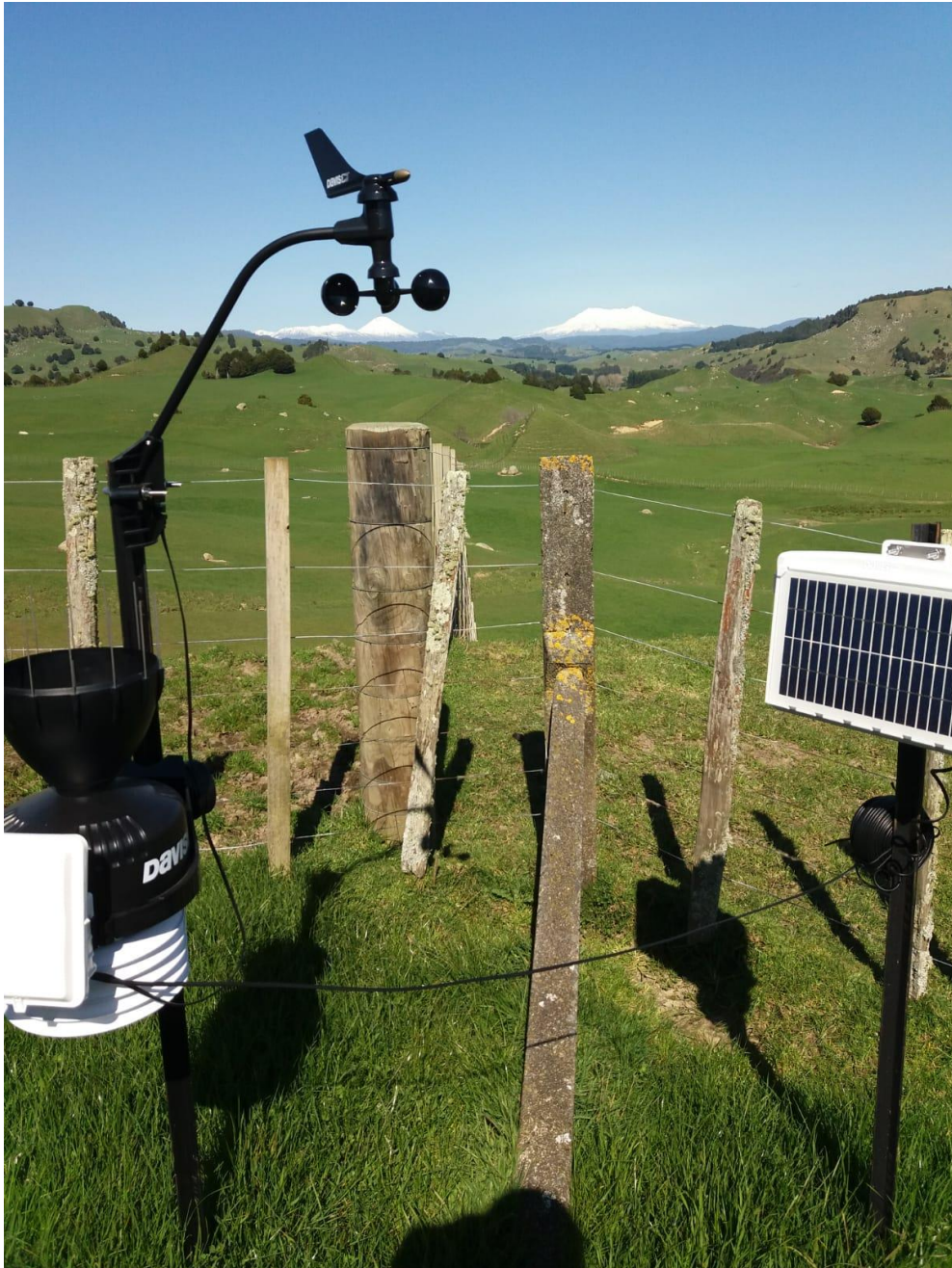
Figure 4.2 The Davis Vantage Pro2 6322C in position on “M” Station, North Island.
