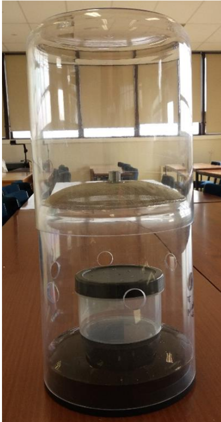
Figure 3.2 The unpainted version of the Western Australian Trap, showing the internal design.
