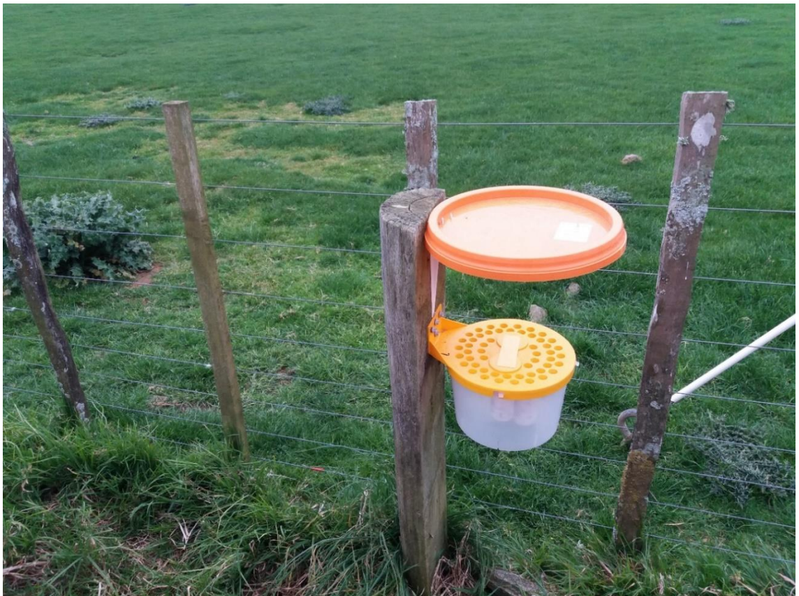
Figure 4.1 Photo illustrating the standardized trap layout used on each of the study farms, a LuciTrap with a StickyTrap adhered to the lid. The LuciTrap was positioned 1.5m in height with a rain deflecting lid above the trap.
